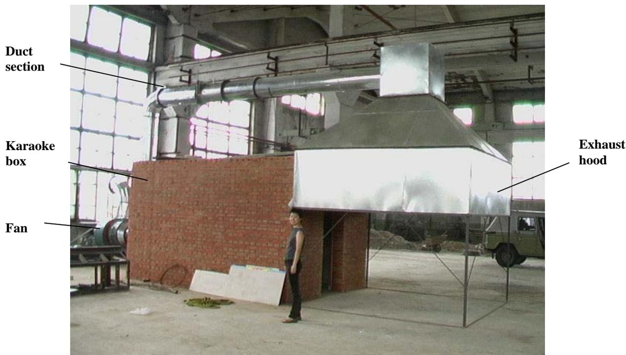
**Fig. 5: Setup for karaoke box fire test at the PolyU/HEU site**
