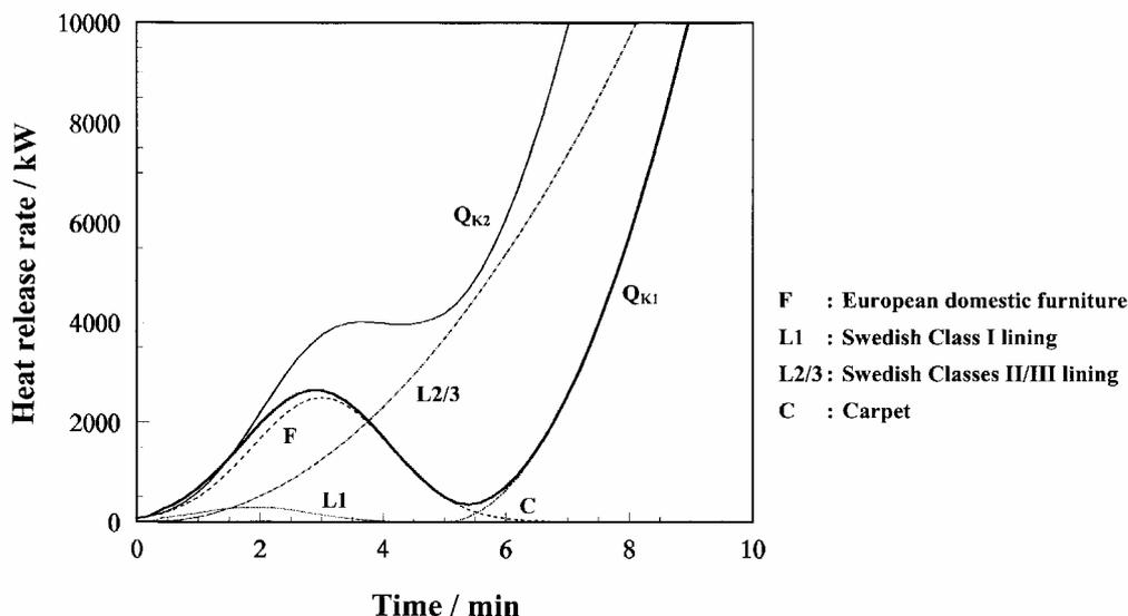
Fig. 1: Example of estimating heat release rate in a karaoke box
