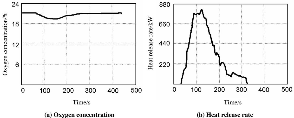
Fig. 6: Typical results on burning diesel
