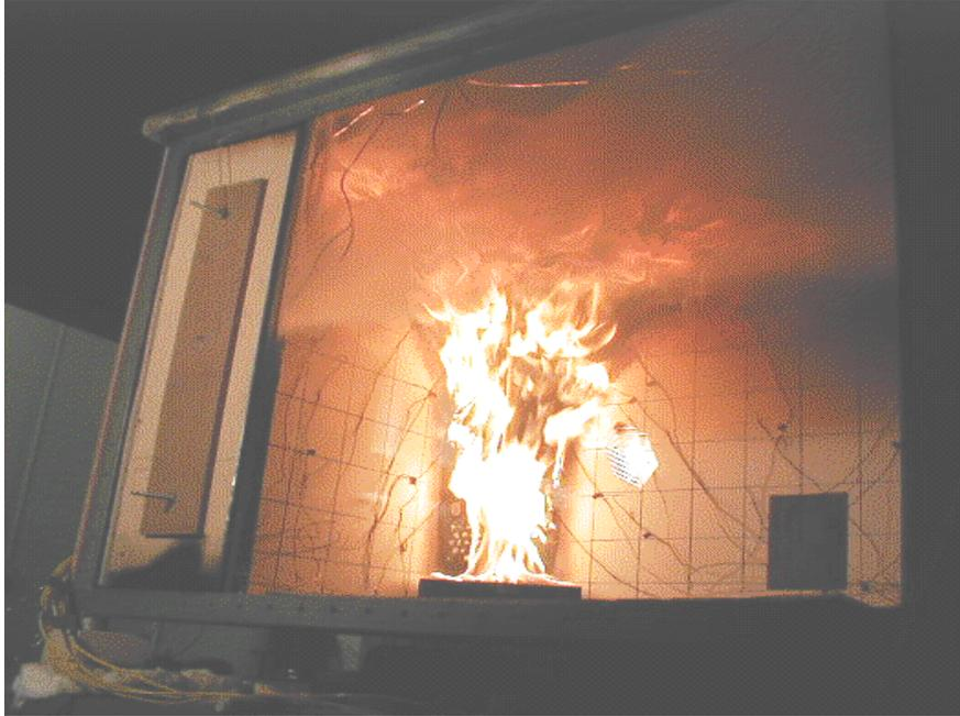
**Fig. 9: Test Compartment B melamine chipboard lining. Developing fire. 50 seconds after ignition of fuel.**
