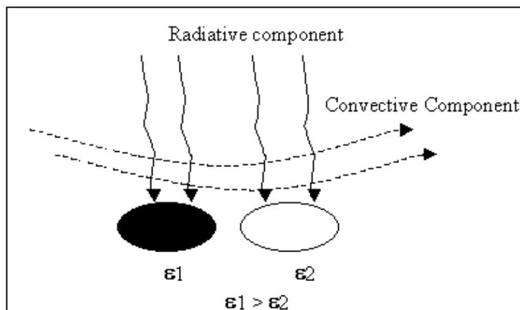
Fig. A1: TPD theoretical principle of operation
