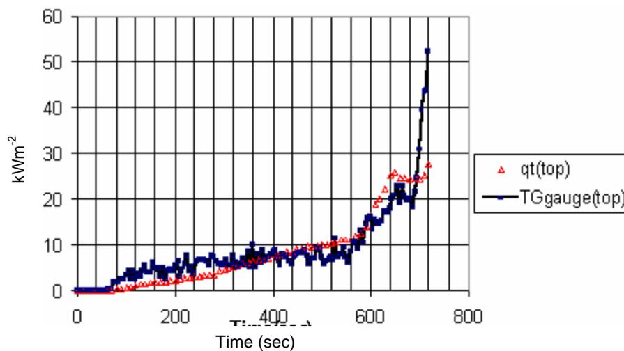
Fig. 12: Corner fire test. Top position. Results employing modified TPD calibration method. Melamine chipboard linings.
