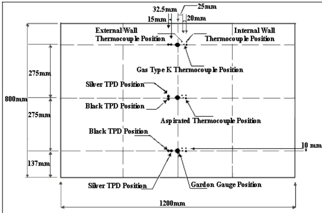
Fig. 2: Front wall instrumentation location Compartment A
