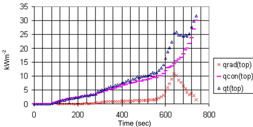
**Fig. 14: Convective to radiative heat flux partitioning employing modified TPD calibration method. Melamine chipboard linings.**
