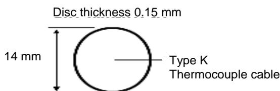
Fig. 1: Thin plate device design
