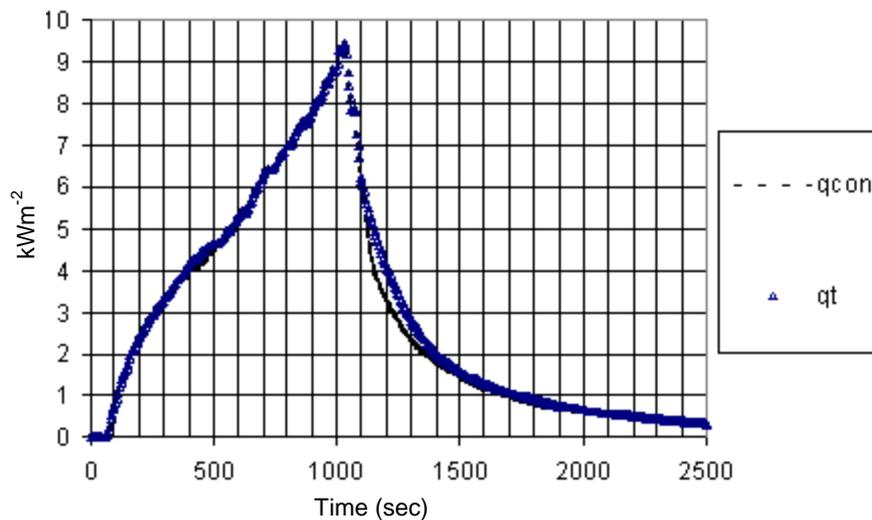
Fig. 15: Fire resistant chipboard Linings. Comparison of convective and Total heat flux.
