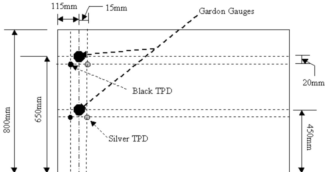
Fig. 4: Rear wall instrumentation location
