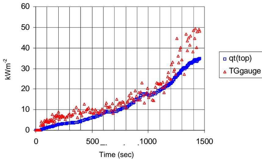
**Fig. 13: Corner fire test. Top position. Fire resistant chipboard. Results employing modified TPD calibration method.**
