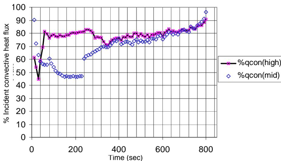
Fig. 8: Convective to total heat transfer ratio for Corner test (Meths fuel)
