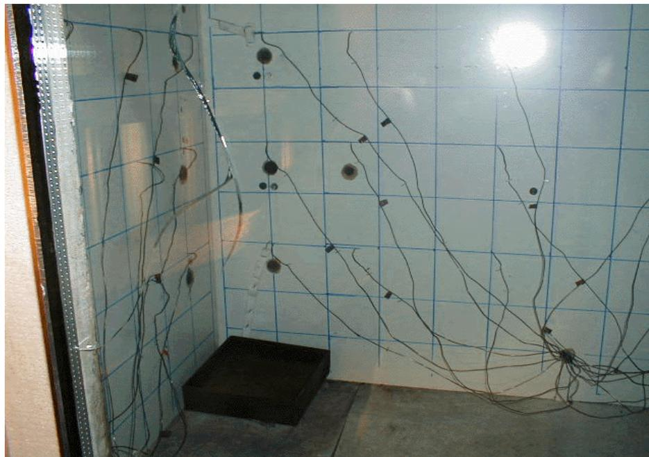
Fig. 3: Compartment B with melamine chipboard linings test set up
