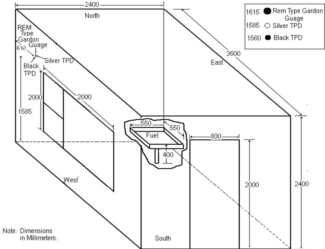
Fig. 5: Full scale ISO test compartment
