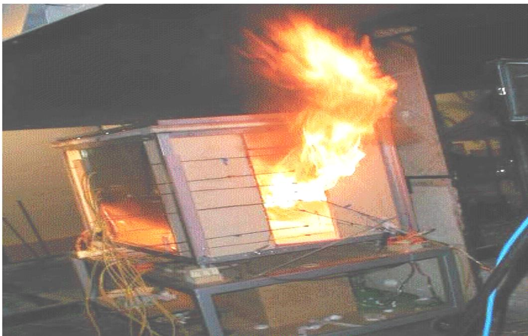
**Fig. 10: Test Compartment B melamine chipboard lining. 600 seconds after ignition of the fuel.**
