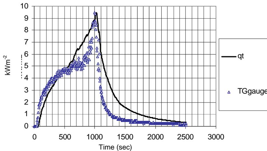
Fig. 16: Fire resistant chipboard linings. West wall beside window. High position. Comparison with Total Gardon Gauge output.
