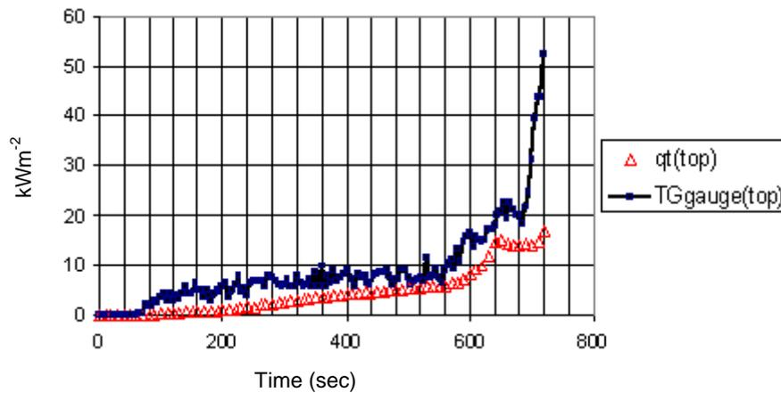
Fig. 11: Corner fire test. Top position. Results employing the initial TPD calibration method. Melamine chipboard linings.
