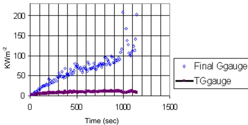
Fig. 6: Corner fire test. Unlined (Meths/Diesel mixture). Corrected total incident flux.
