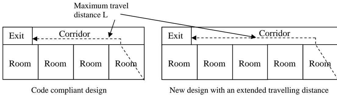
Fig. 1: Schematic layout of a code compliant design and a new design
