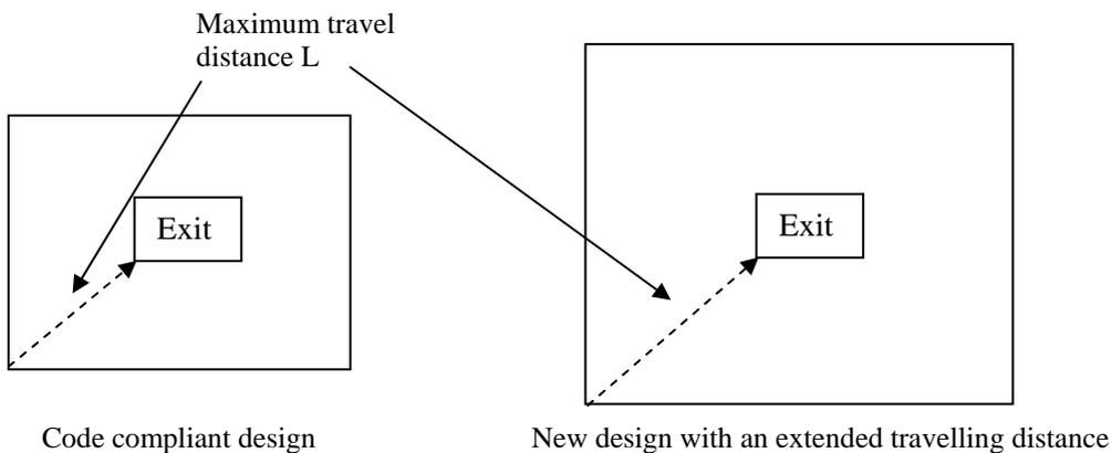
Fig. 2: Schematic layout of a code compliant design and a new design
