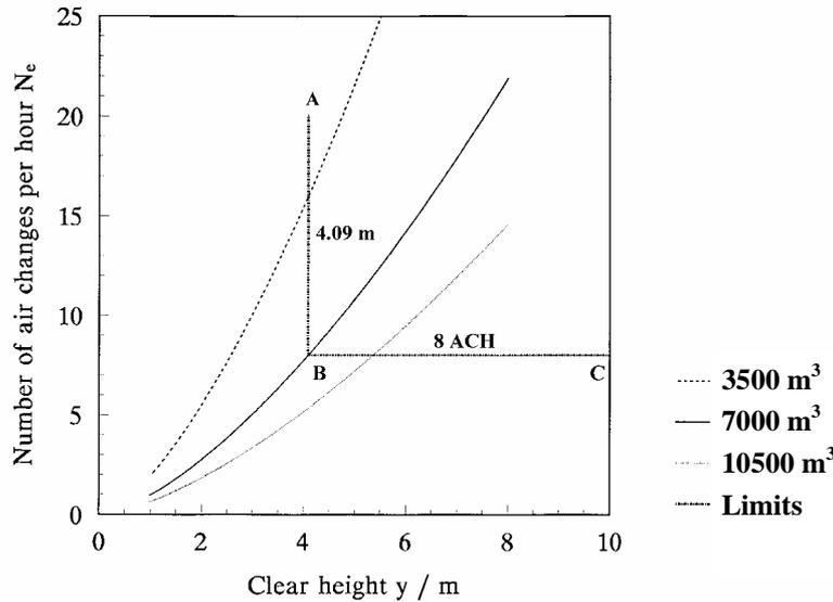
Fig. 1: Extraction rates at different clear heights
