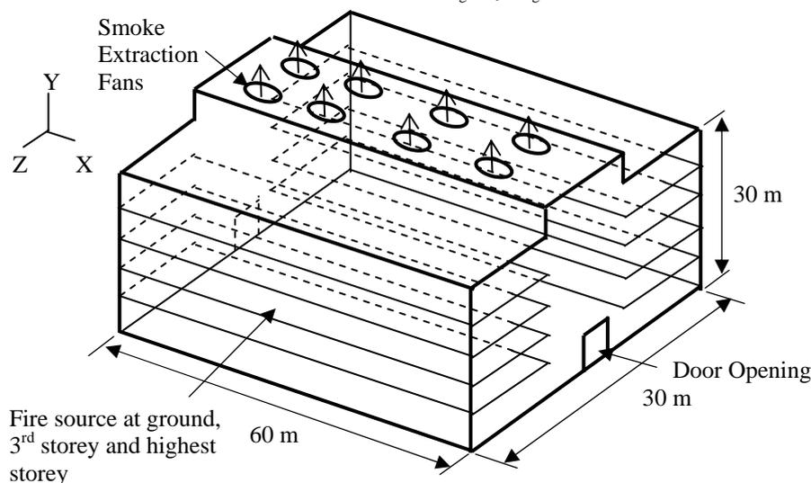
Fig. 1: Geometry of numerical experiment NA
