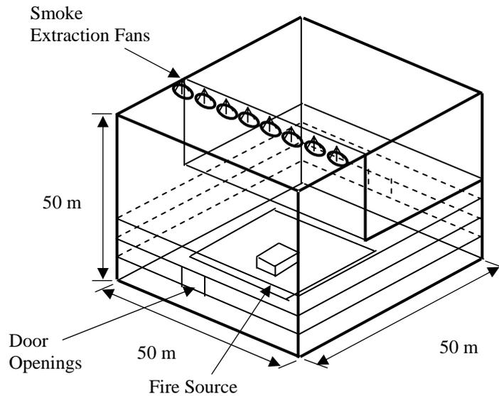
Fig. 3: Geometry of the physical model PM
