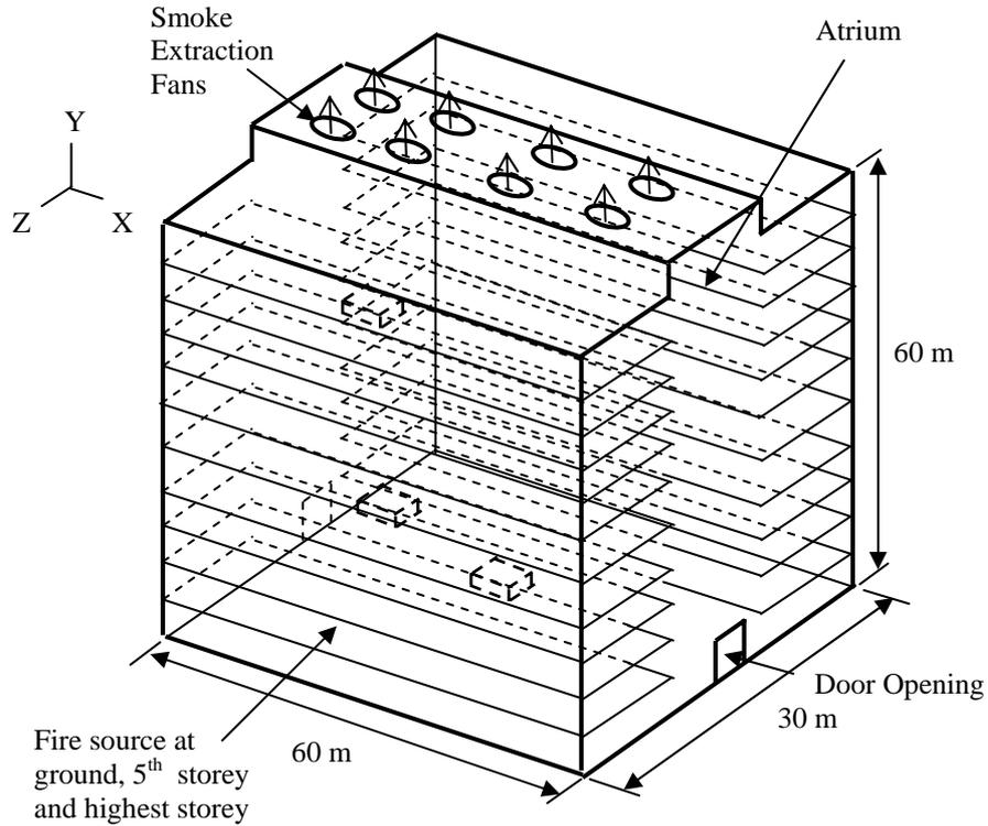
Fig. 2: Geometry of numerical experiment NB
