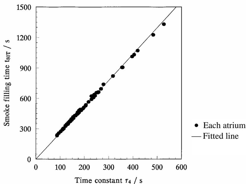
Fig. 1: Time to fill 80% of atrium with smoke
