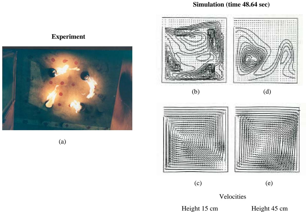
**Fig. 3: Comparison of experimental observation and simulated results at large D (D = 60 cm experimental, D = 51 cm simulation)**
