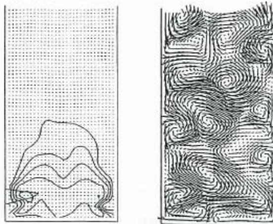
**Fig. 9: Vertical section temperature and velocity fields for Case 7**
