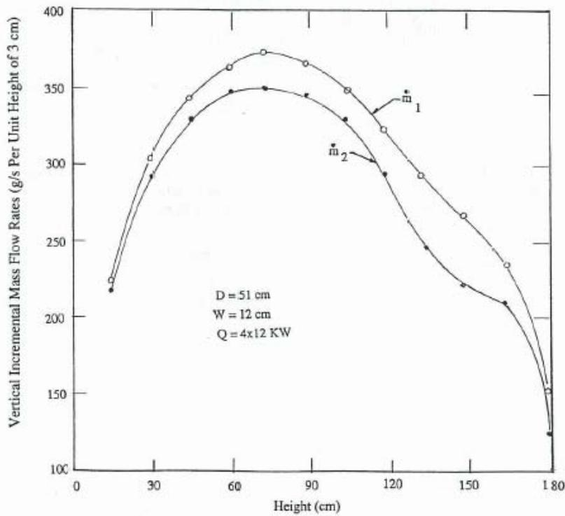
Fig. 6: Incremental mass flow rates  $\dot{m}_1$  (upward flow) and  $\dot{m}_2$  (downward flow) at different heights
