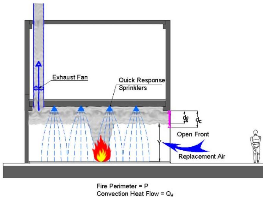
Fig. 1: The SHEVS Cabin-Principle – section through cabin
