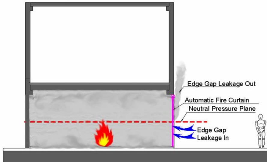
Fig. 4: The Depressurised Cabin-Principle – without depressurisation – section through cabin
