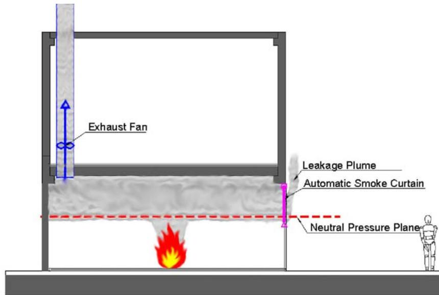
Fig. 2: The SHEVS Cabin-Curtain edge leakage – section through cabin
