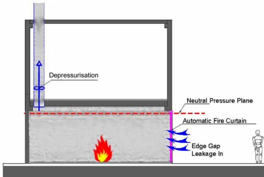
Fig. 5: The Depressurised Cabin-Principle – with depressurisation – section through cabin
