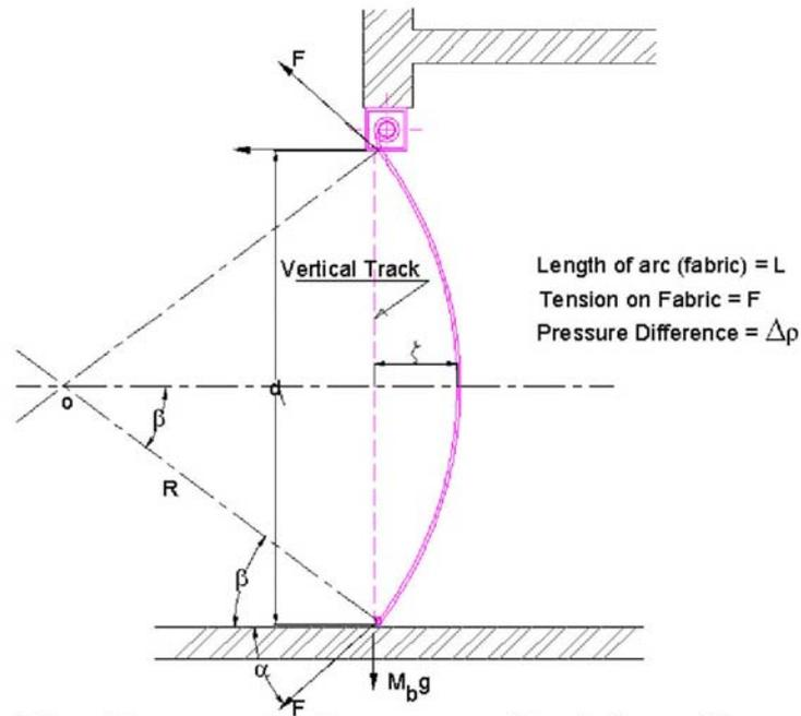
Fig. 6: The forces acting on a curtain with constrained bottom bar - section
