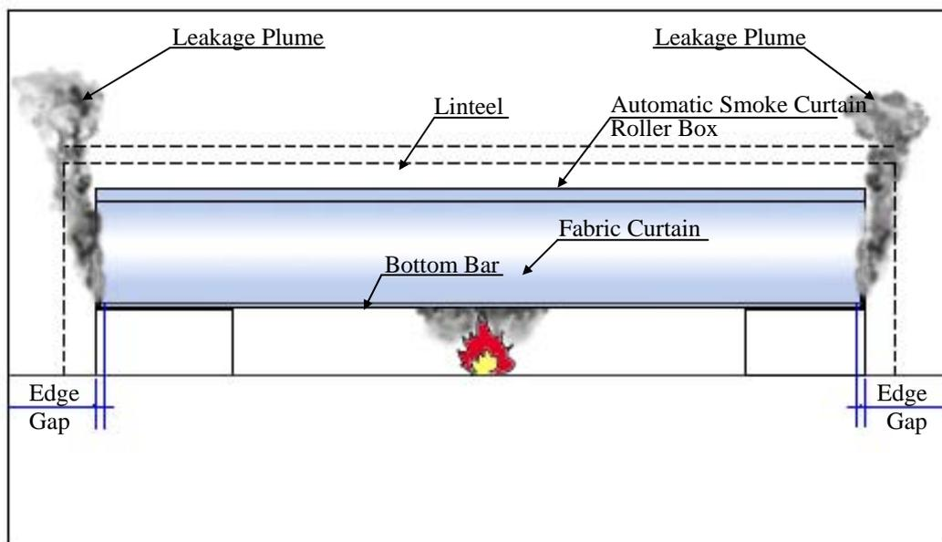
Fig. 3: The SHEVS Cabin-Curtain edge leakage – front view of cabin
