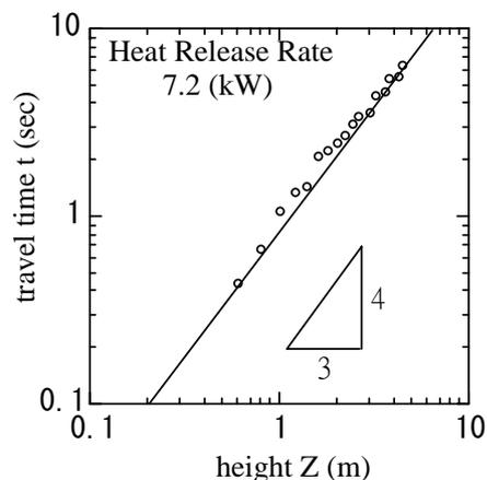
Fig. 11: Travel time versus height from fire source
