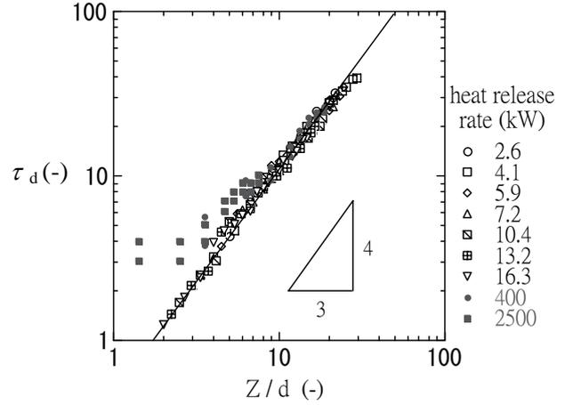
Fig. 12: Non-dimensional travel time  $\tau_d$  in free spaces (characteristic length  $d$ )
