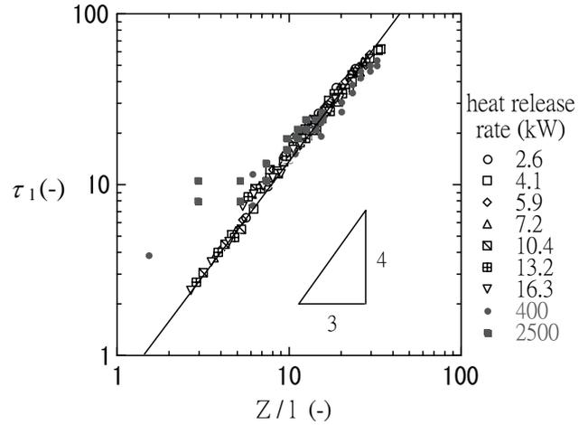
Fig. 13: Non-dimensional travel time  $\tau_l$  in free spaces (characteristic length  $l$ )
