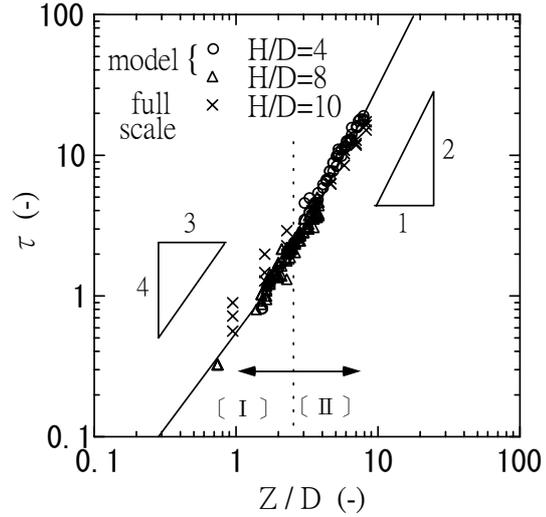
**Fig. 15: Non-dimensional travel time  $\tau$  in closed shafts**
