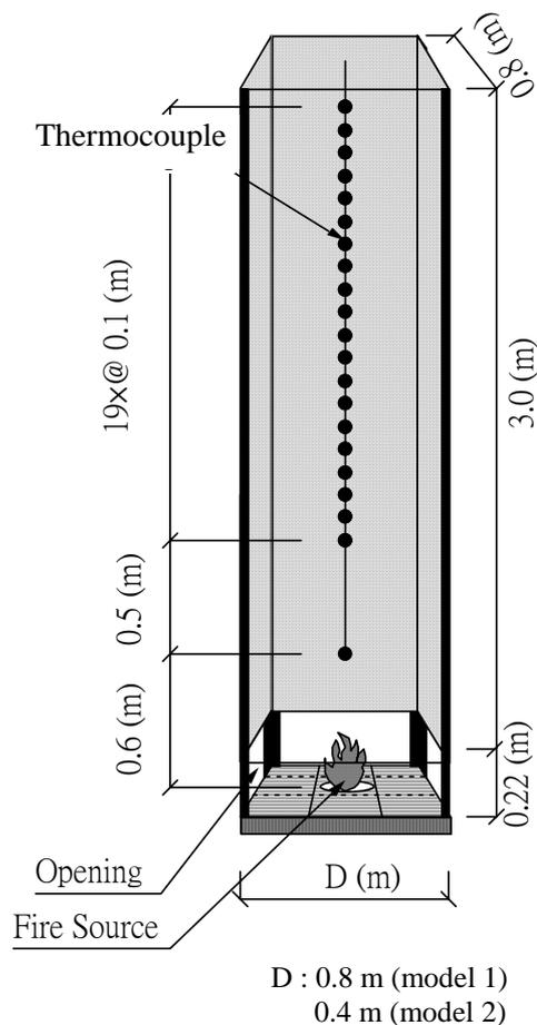
Fig. 4: Setup and geometrical conditions of reduced scale shaft
