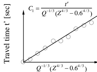
Fig. 10: Modified travel time and experimental coefficient
