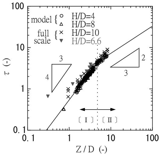
**Fig. 14: Non-dimensional travel time  $\tau$  in open shafts**
