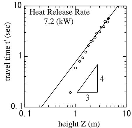
Fig. 9: Travel time from the lowest thermocouple in a reduced scale free space test
