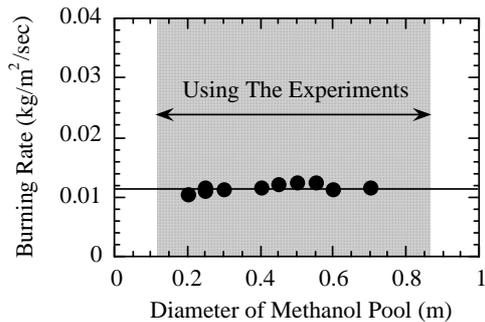
**Fig. 2: Burning rate of methanol pool with different diameter [8,9]**
