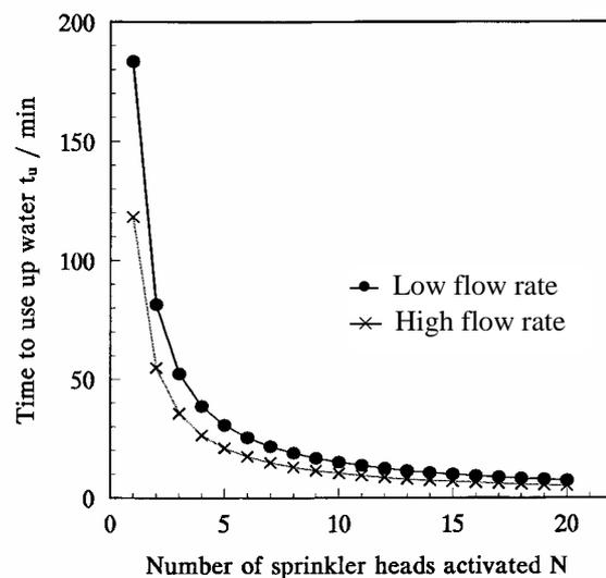
**Fig. 1: Time to use up water in the tank**
