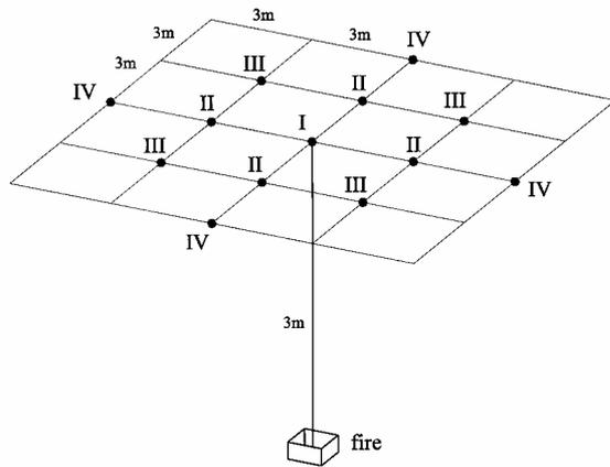
Fig. 2: Geometry of layout of sprinklers
