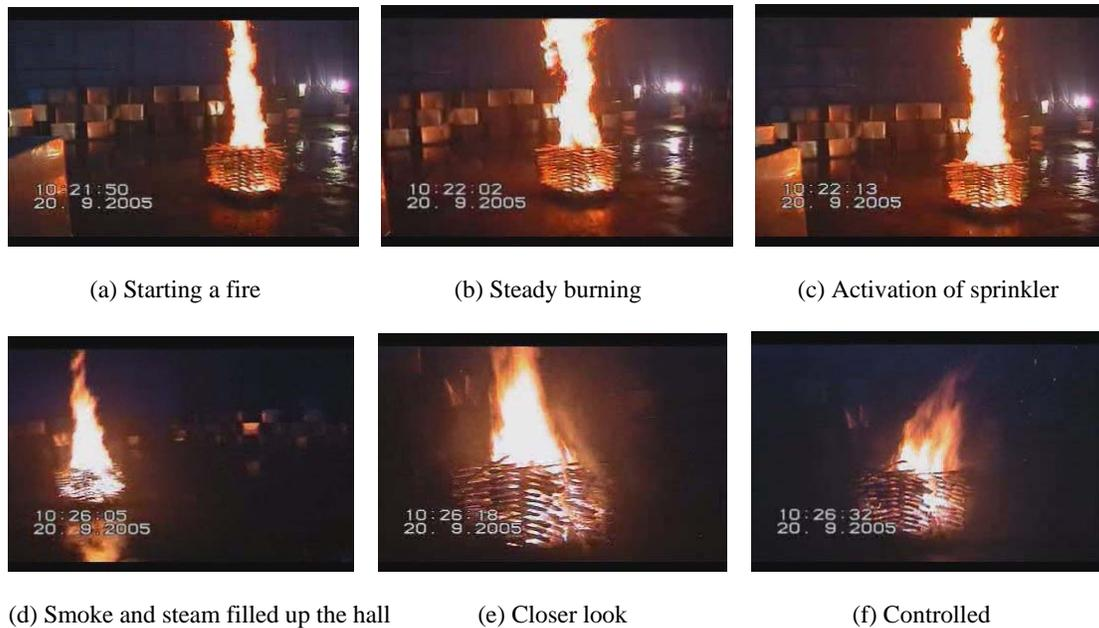
**Fig. 3: Action of long-throw sprinkler on a small 0.5 MW wood crib fire**
