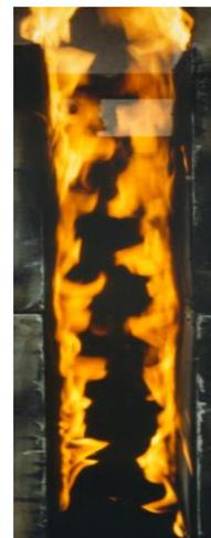
**Fig. 1: Instantaneous view of the burning between parallel vertical walls from a video camera**
