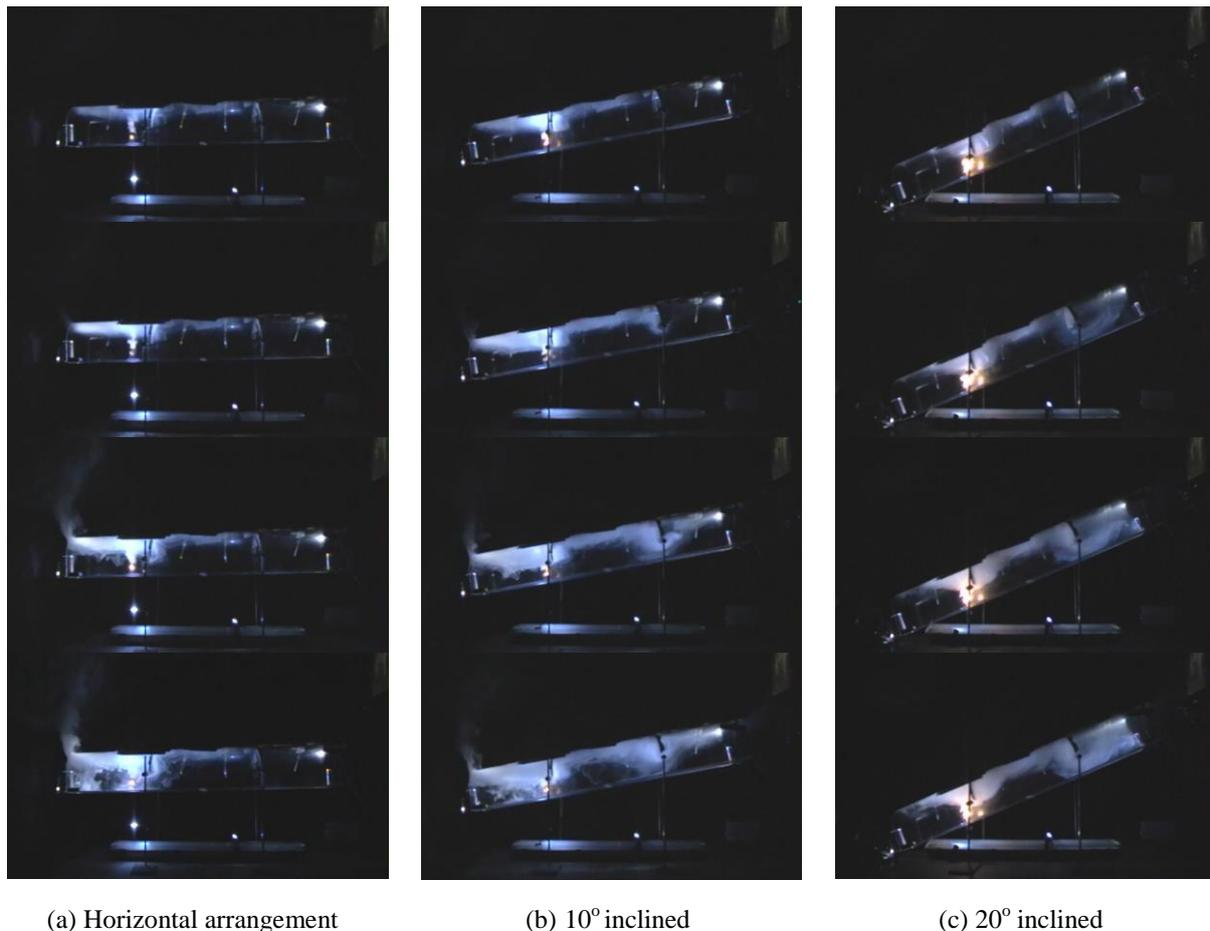
**Fig. 1: Smoke movements inside the tunnel with smoke barrier**
