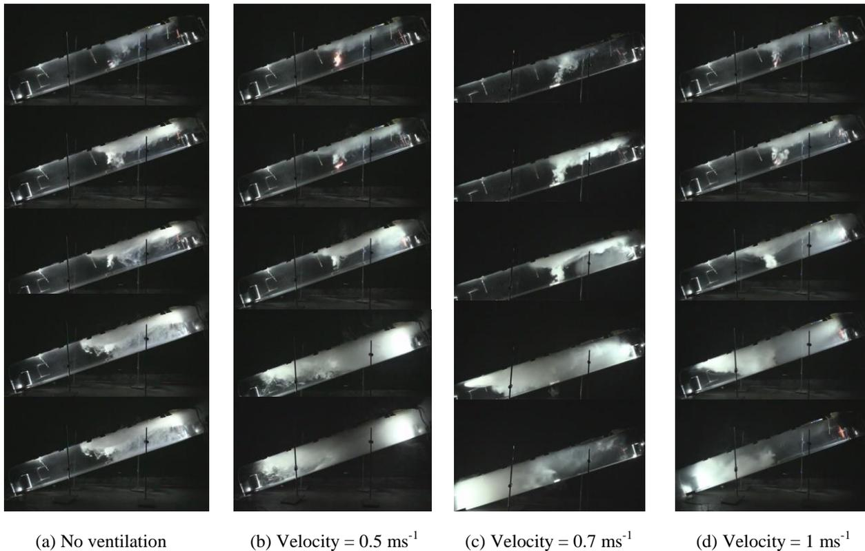
**Fig. 4: Smoke movements inside the tunnel inclined at 20°**
