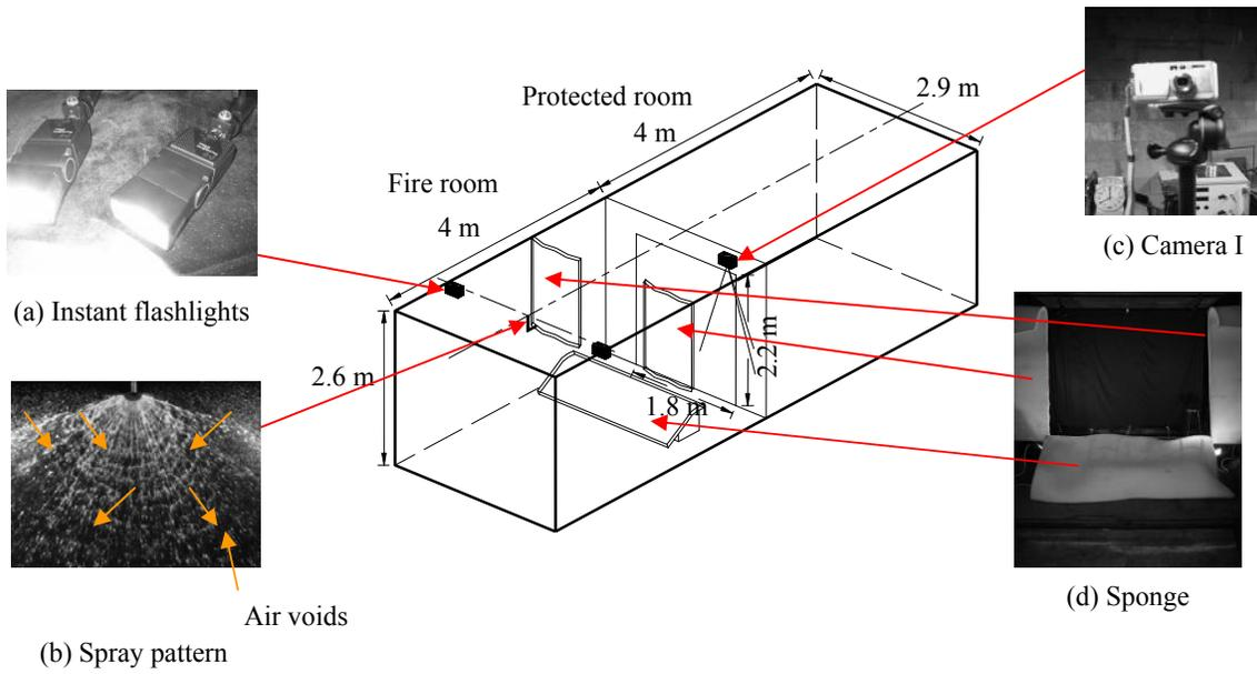
Fig. 1: Experimental setup for taking photographs
