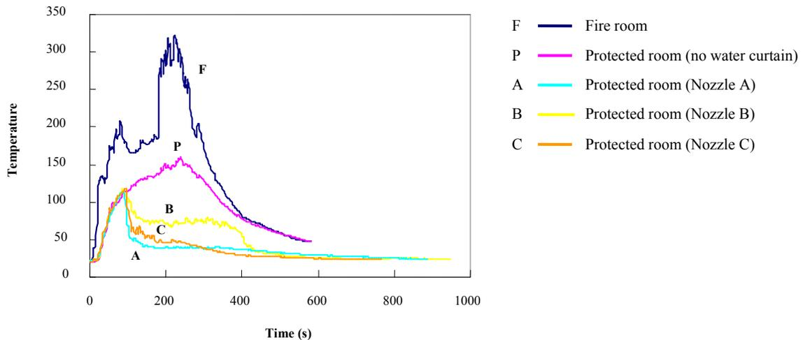
Fig. 4: Temperature profile in the two chambers
