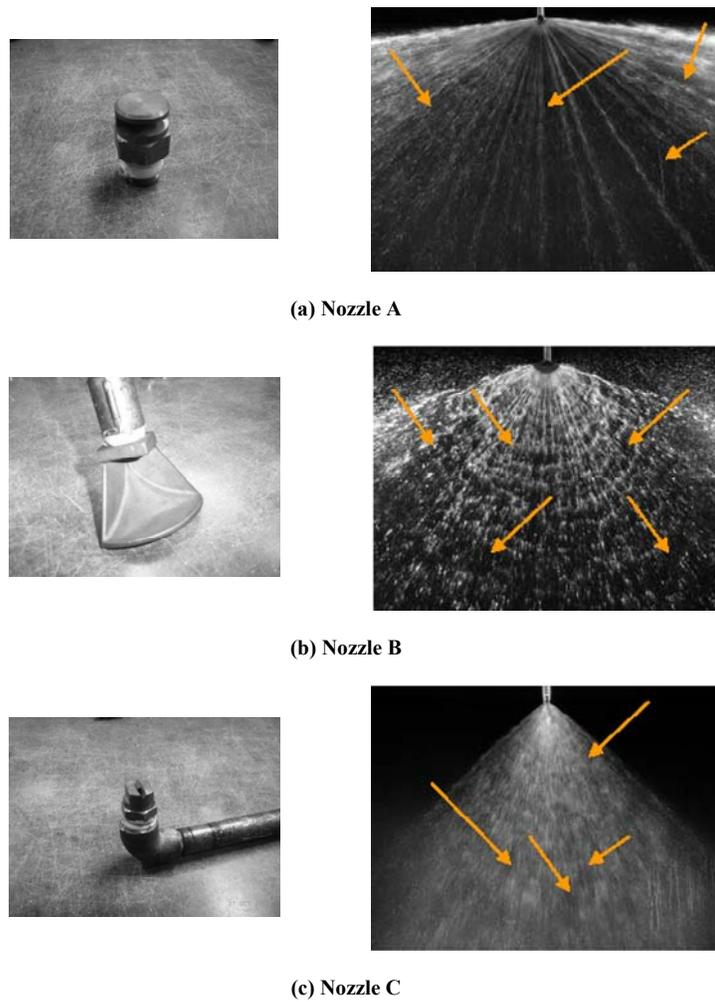
Fig. 2: The three tested nozzles
