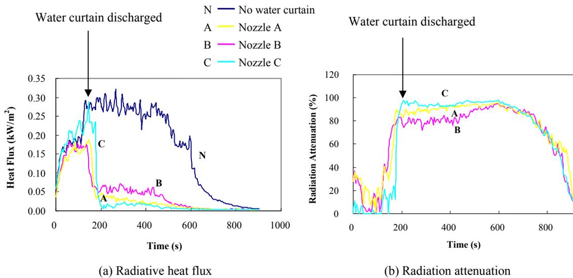
Fig. 3: Radiation blockage
