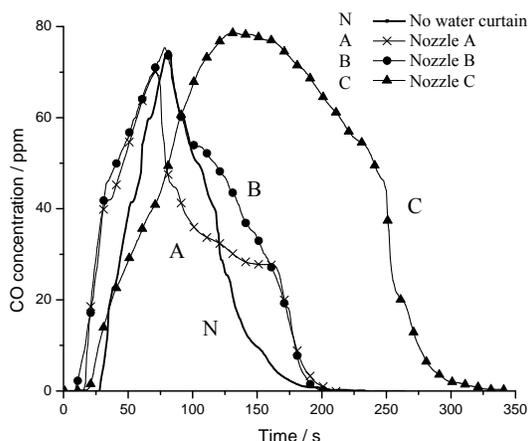
**Fig. 5: CO concentration during fire with and without discharging water curtain**
