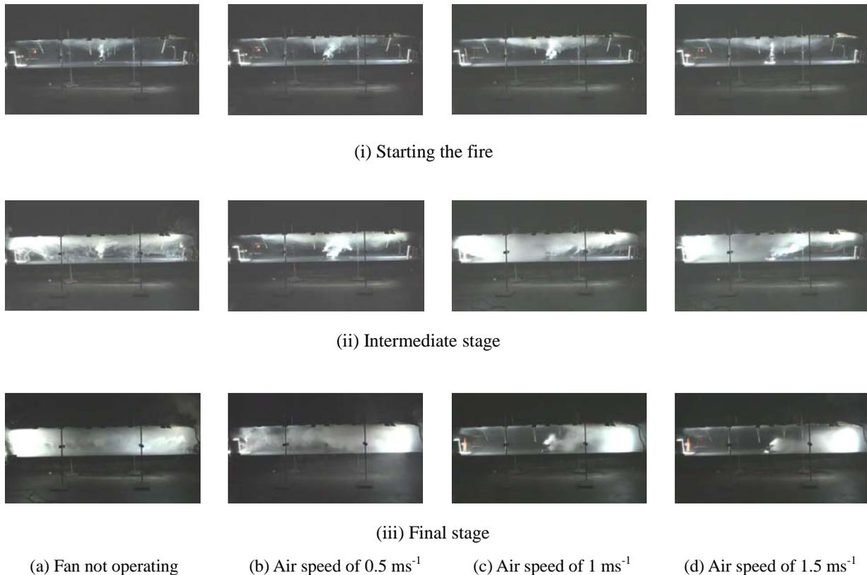
**Fig. 2: Typical smoke movements pattern**
