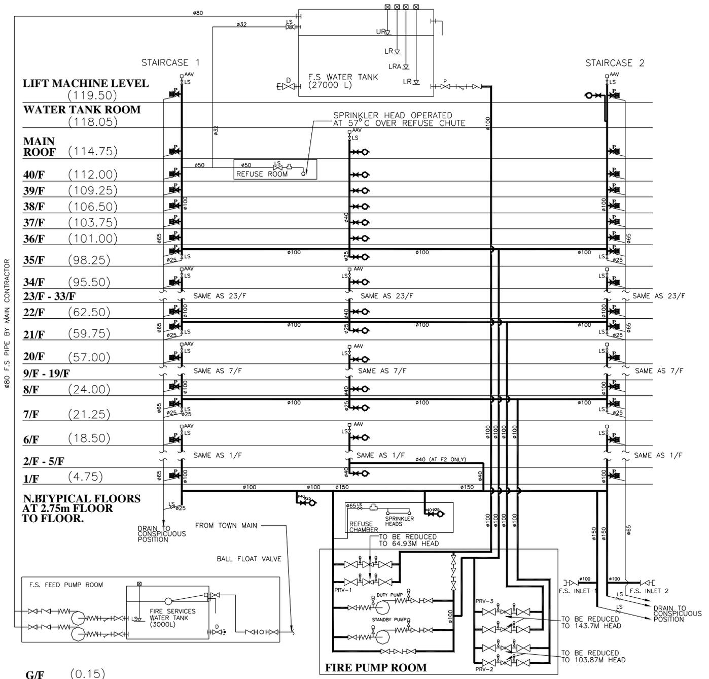
Fig. 5: Schematic diagram for fire hydrant / hose reel system of a supertall building
