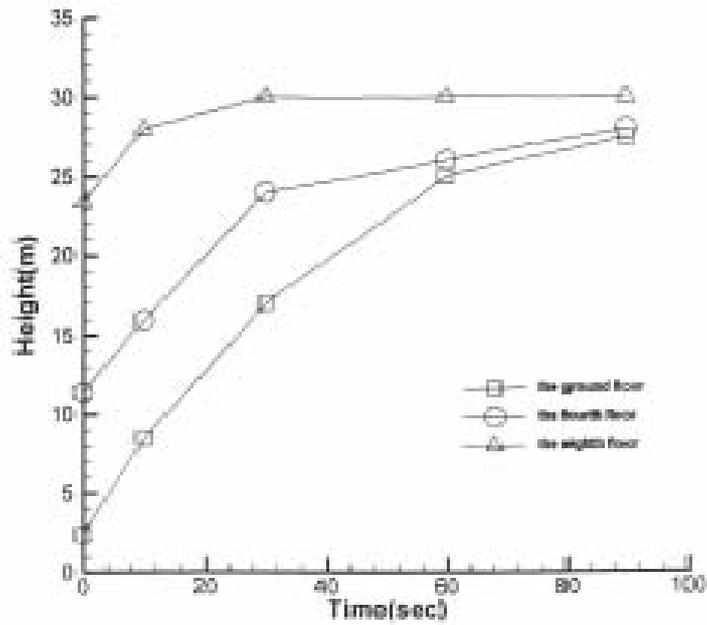
Fig. 5: The effect of floor level on smoke temperature transportation inside a smoke exhaust duct
