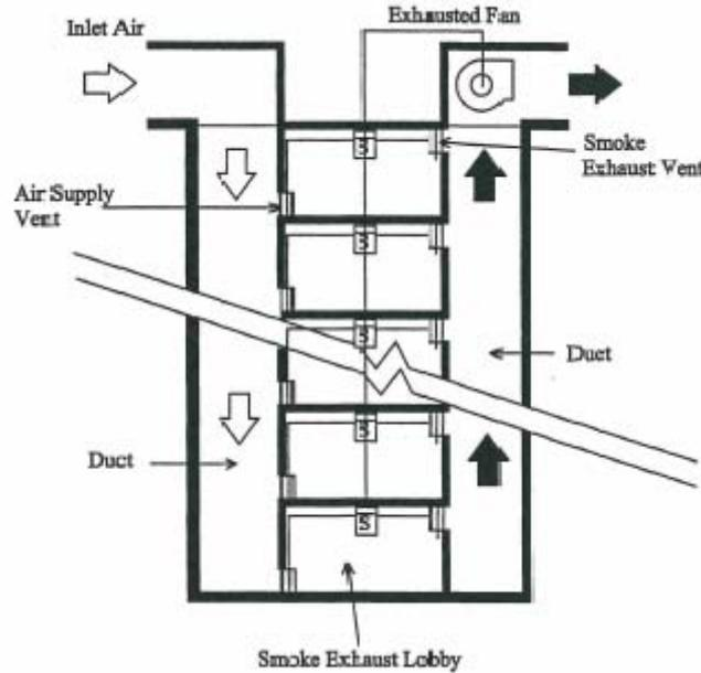
**Fig. 2: Description of the mechanical ventilated smoke control system in a tall building with air supply and smoke exhaust vents**
