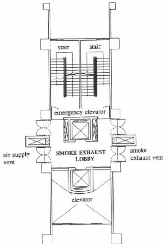
**Fig. 1: A typical smoke exhaust lobby design of tall buildings in Taiwan area**
