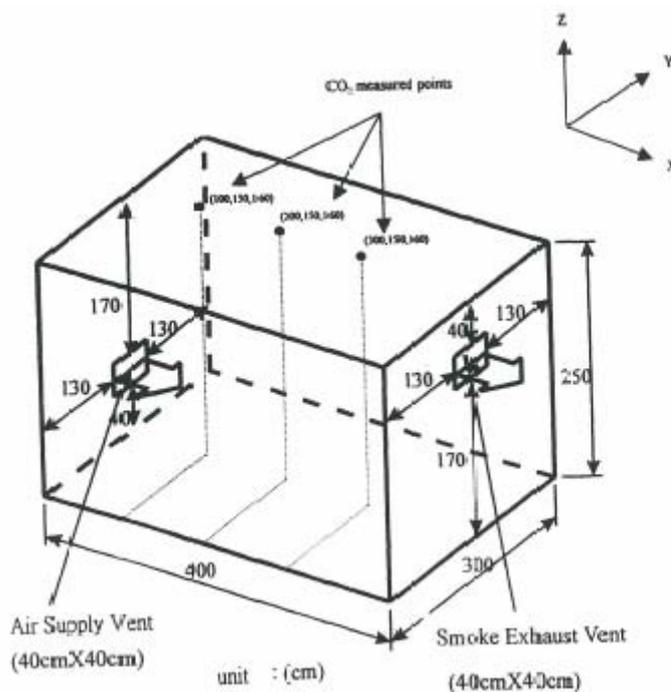
Fig. 3: Model smoke exhaust chamber used for full-scale experiments and simulations
