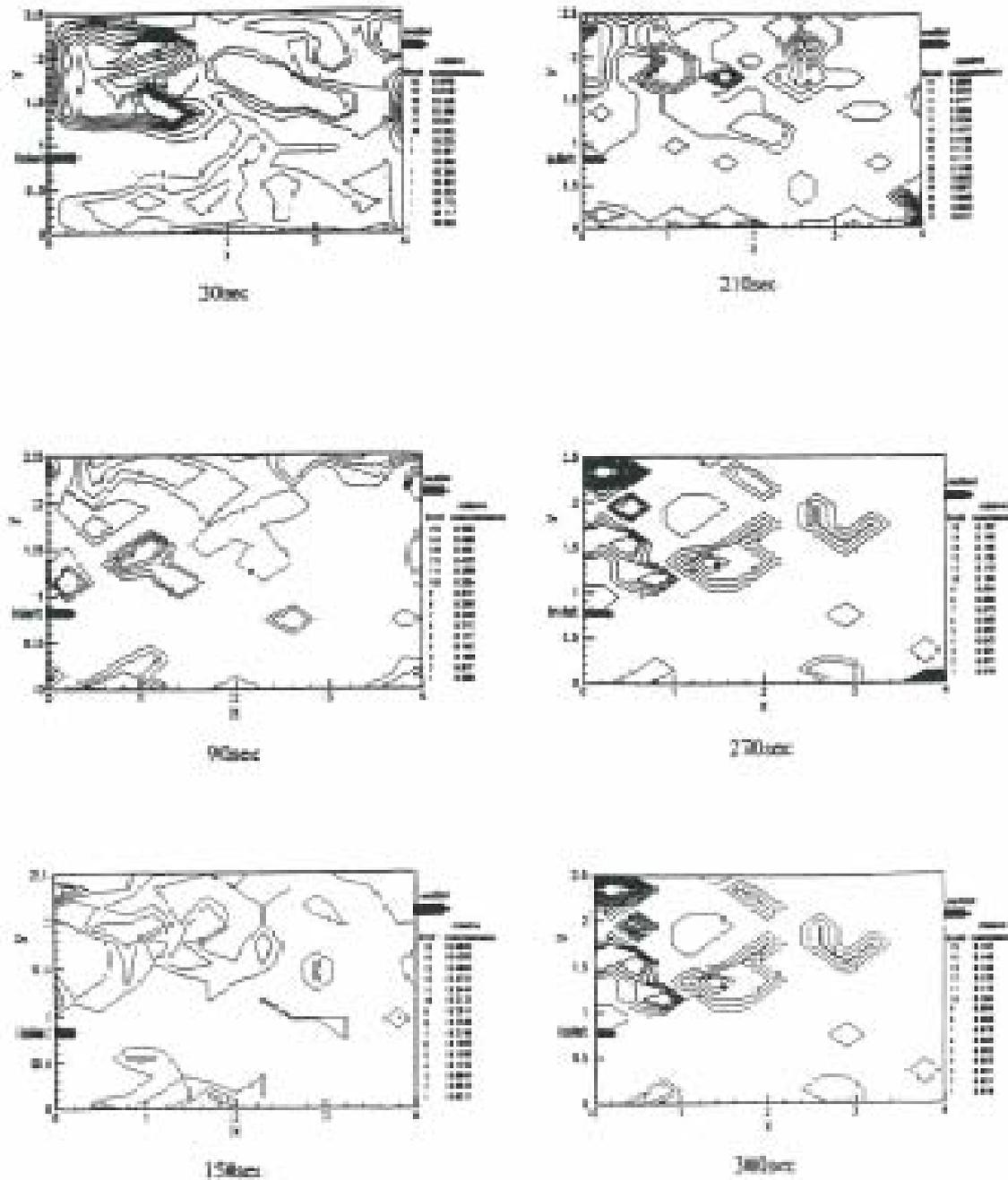
Fig. 7: Computed smoke concentration contours of smoke exhaust chamber at  $z = 1.5$  m for x-y plane with different time
