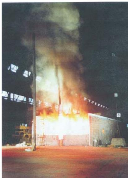
Fig. 10: Test 4: Fully developed fire, 1/2 ventilation
