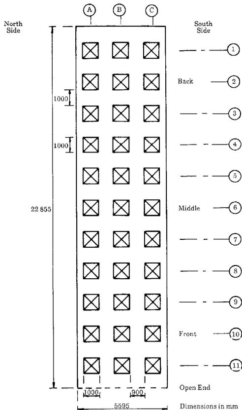
**Fig. 3: Compartment plan showing the layout of the cribs with the back, middle and front measuring stations**
