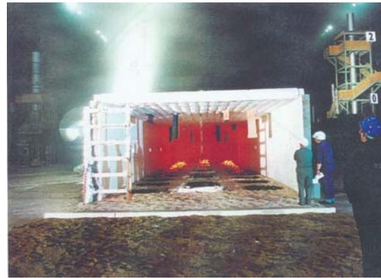
Fig. 12: Complete combustion of the fire loading
