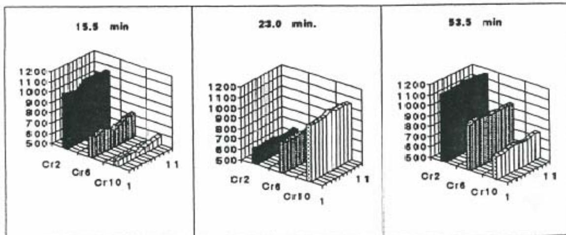
**Fig. 8: Test 2: Horizontal temperature profiles of the hot gases on the crib lines 2, 6 and 10**
