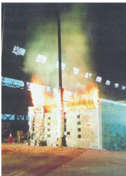
Fig. 11: Test 6: Fully developed fire, 1/8 ventilation
