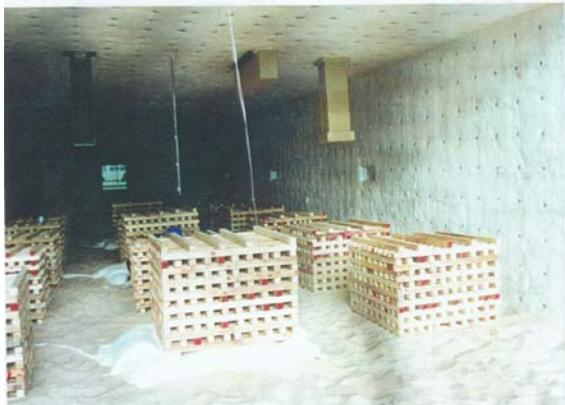
**Fig. 4: Construction of the timber cribs**
