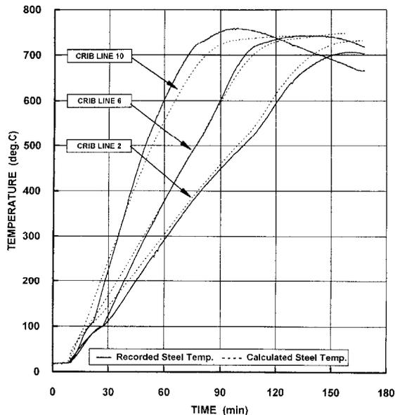
Fig. 14: Comparison between the recorded and calculated heating curves for the protected beams in Test 4
