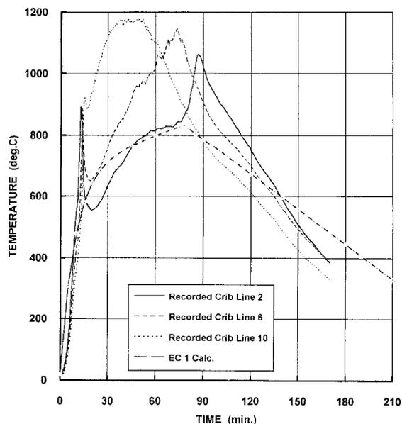
Fig. 15: Comparison of atmospheric heating cycles between measured behaviour and calculated responses using the eurocode parametric relationship
