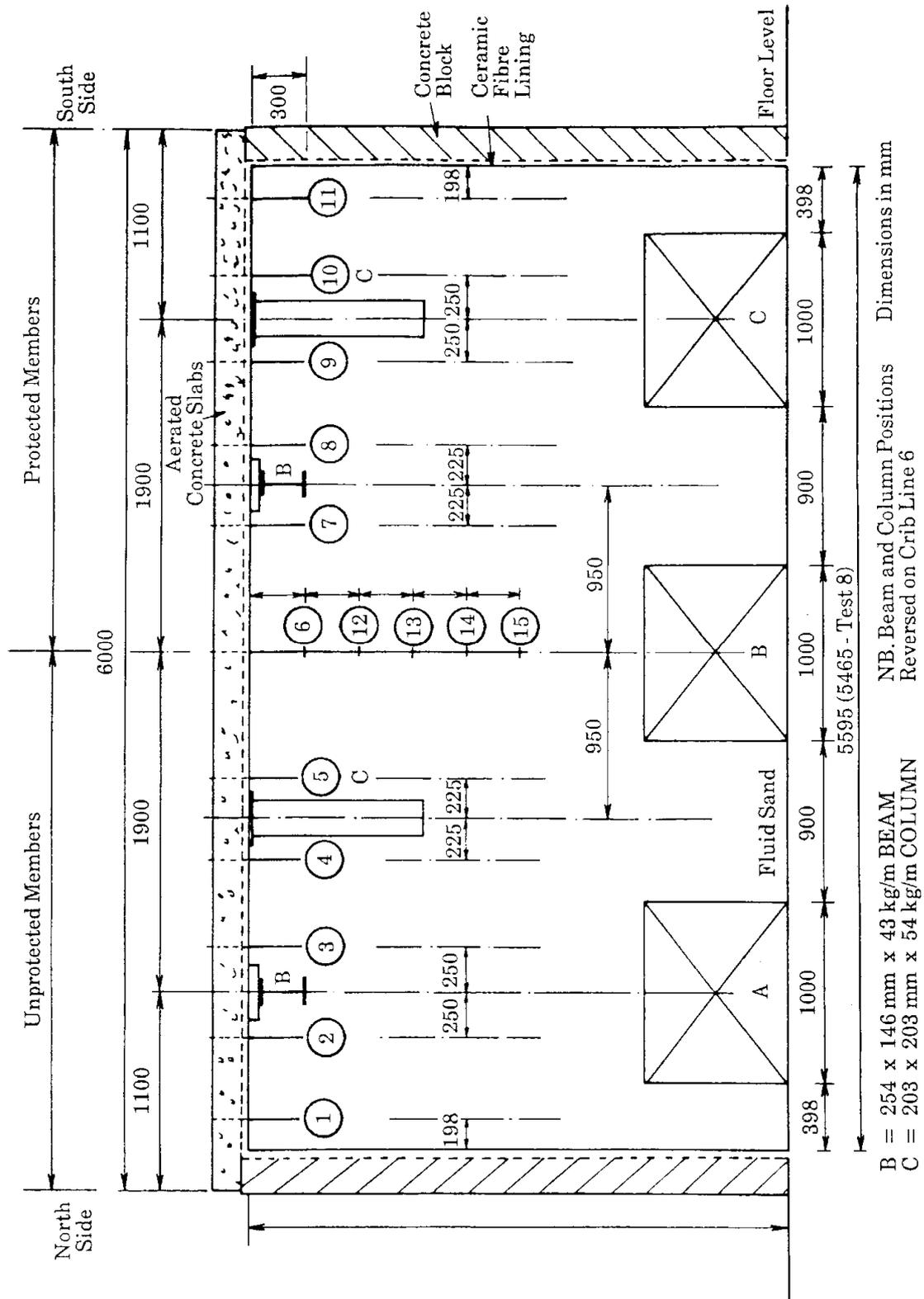
Fig. 5: Section through the compartment on crib lines 2, 6 and 10 showing the position of steel members and thermocouple locations
