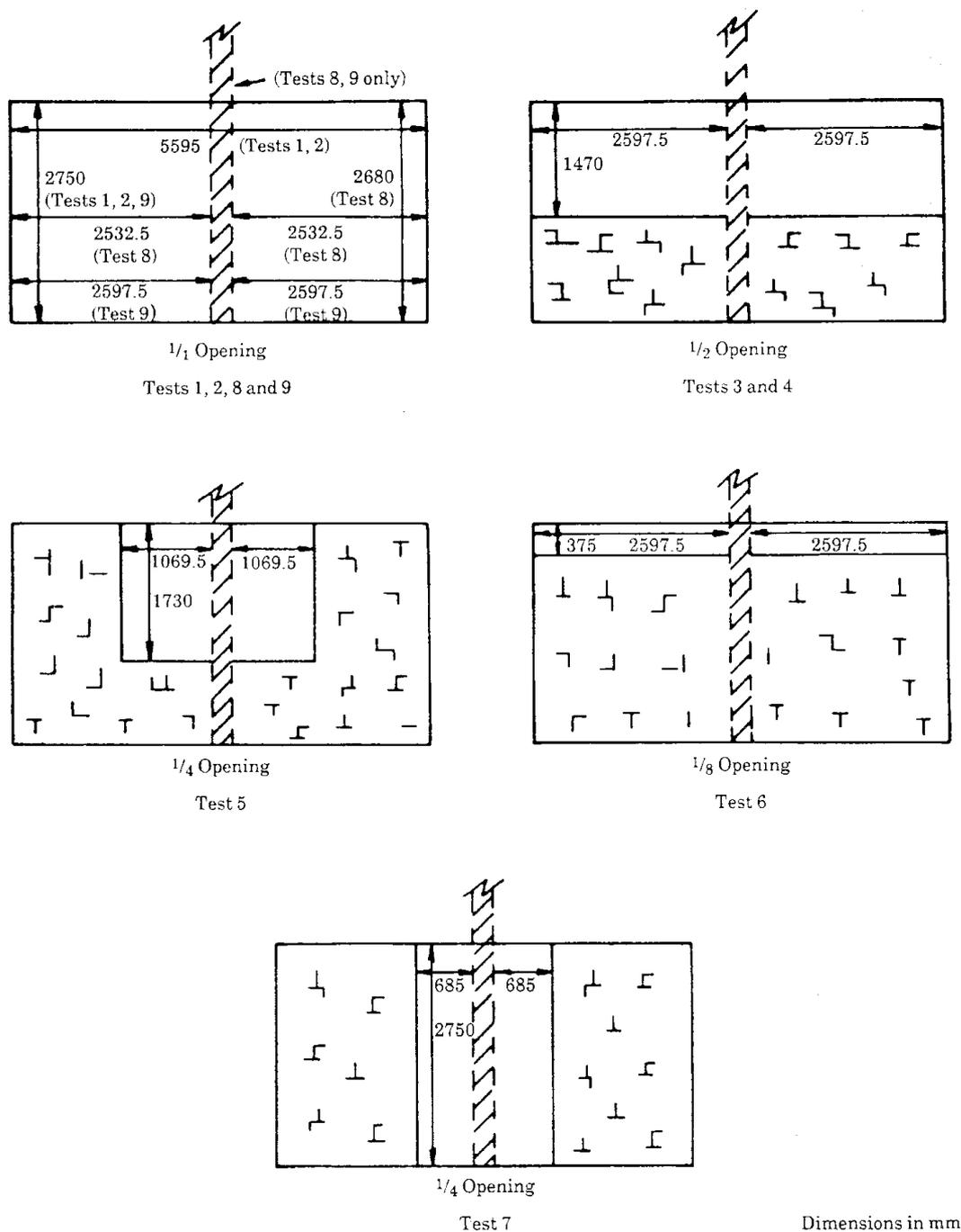
Fig. 2: Dimensions of the ventilation opening conditions
