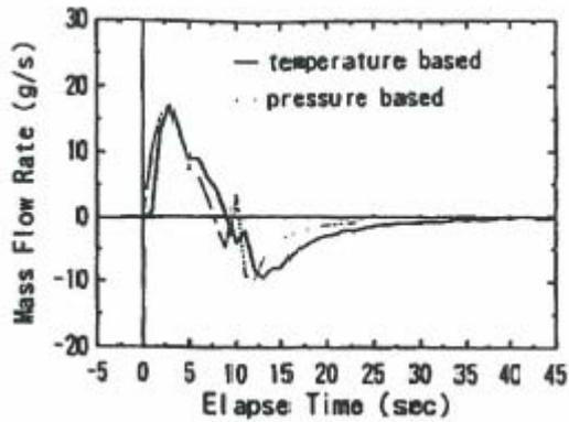
Fig. 5: Estimated mass flow rates based on temperature measurement and pressure measurement
