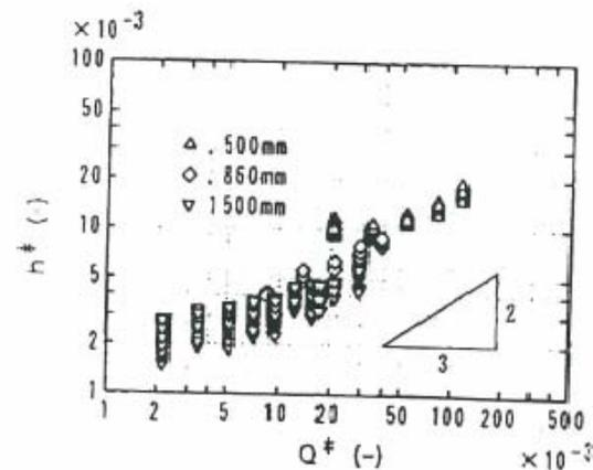
Fig. 9: Relationship between non-dimensional heat release rate and non-dimensional convective heat transfer coefficient (during heat releasing)
