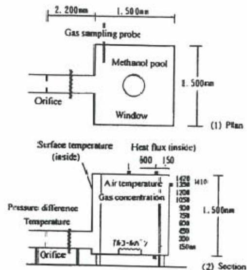
Fig. 1: Schematic of apparatus (medium compartment)
