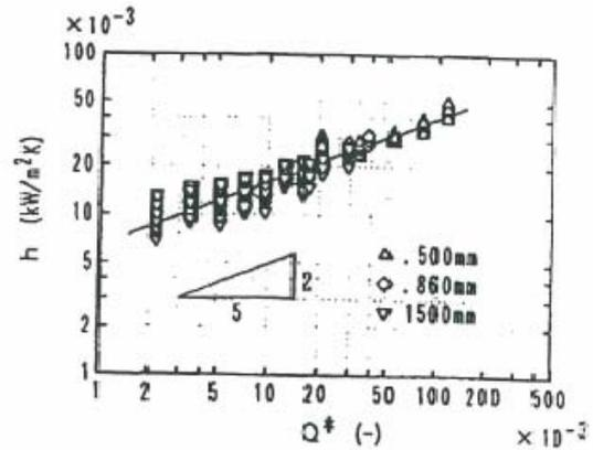
Fig. 8: Relationship between non-dimensional heat release rate and convective heat transfer coefficient
