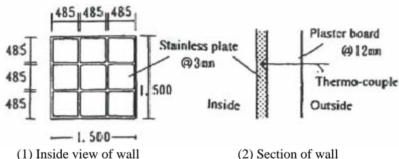
Fig. 2: Stainless plate and thermocouple
