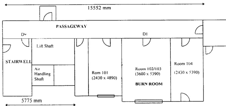
Fig. 2: Level 1 layout of the experimental building-fire facility
