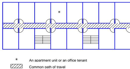
**Fig. 1: Schematic floor layout with a common path of travel**
