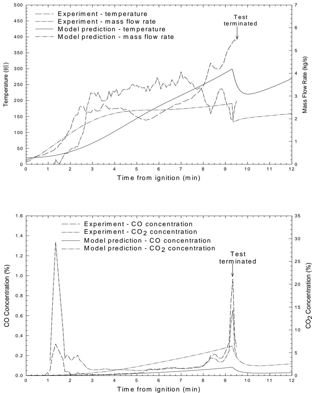
Fig. 2: Comparison of experimental results with model predictions in an open office arrangement
