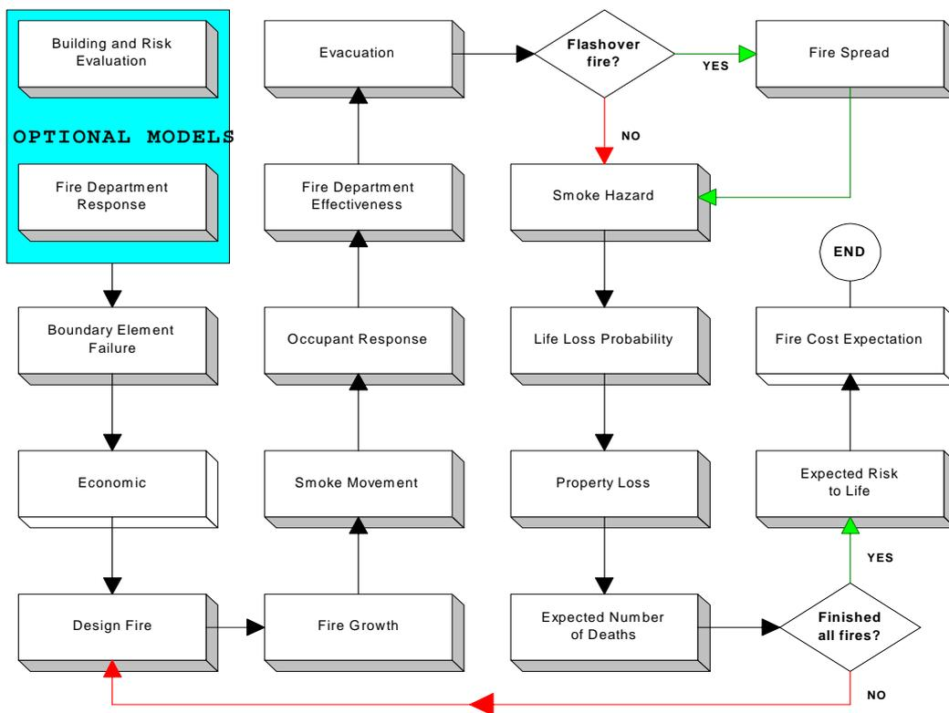
**Fig. 1: FiRECAM™ flowchart**
