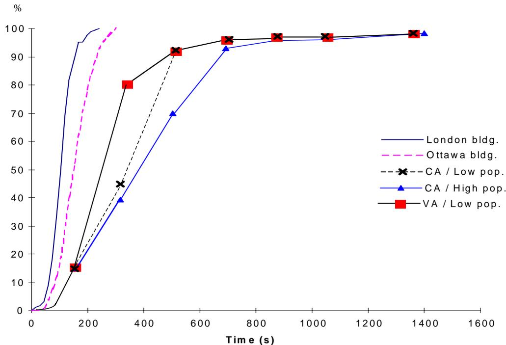
Fig. 4: Comparison of model predictions with results of fire drills in office buildings
