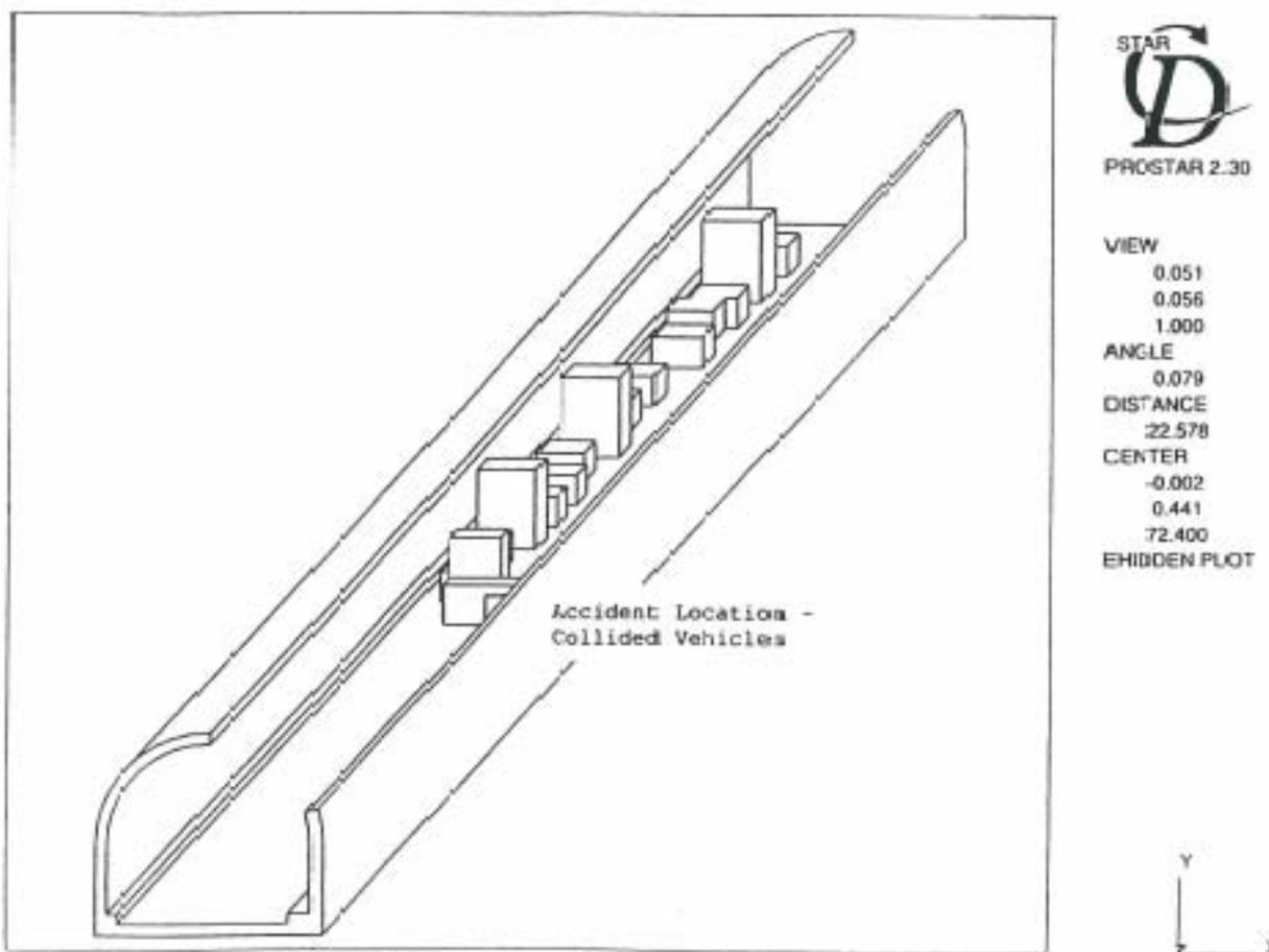
Fig. 2: A three dimensional view across the incident site of the CFD model
