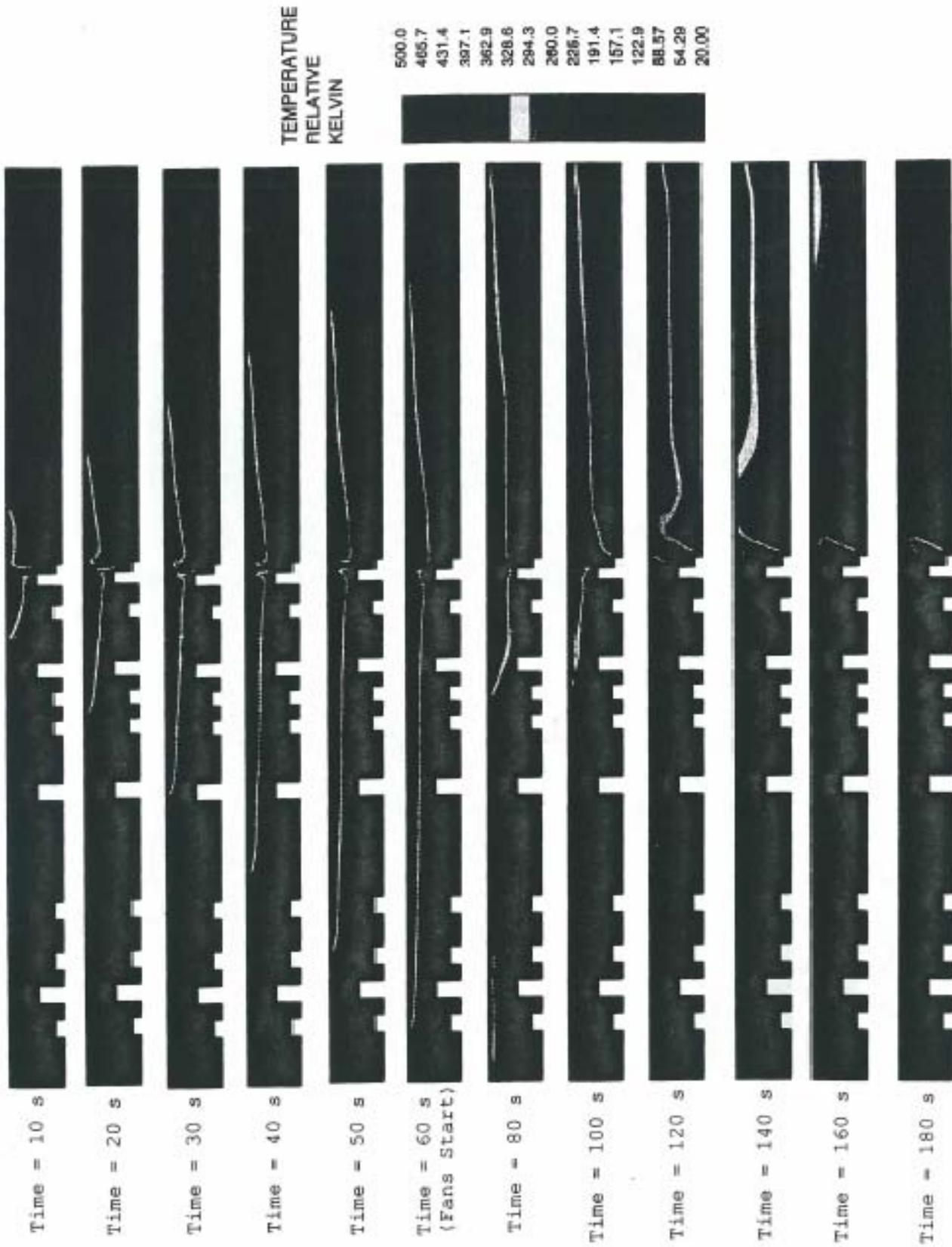
Fig. 4: Transient temperature profile along the tunnel after the car accident
