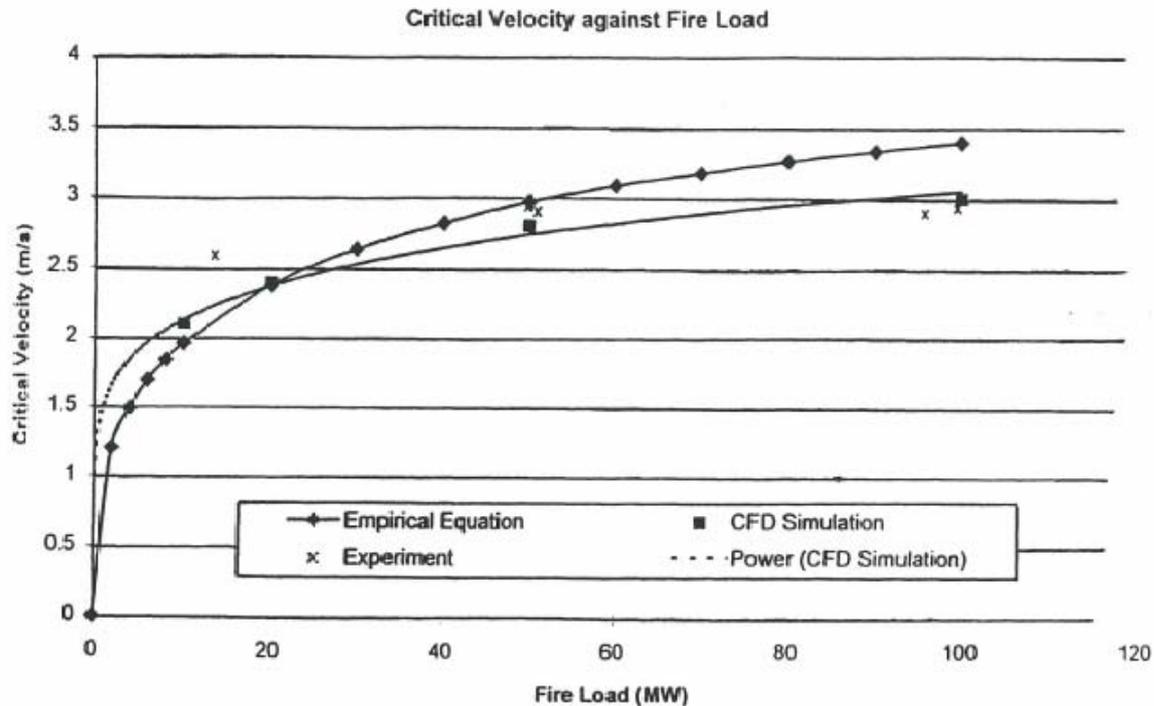
Fig. 1: Critical velocity against fire load
