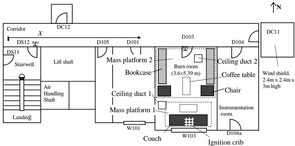
(a) Instrumentation and layout of the first floor
