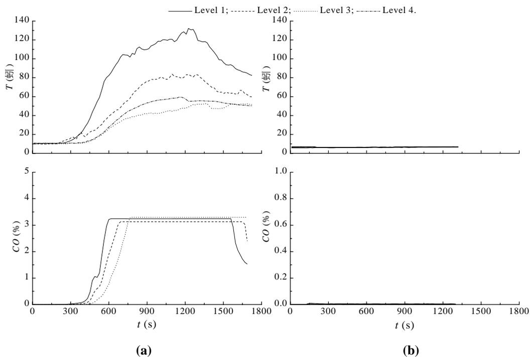
**Fig. 5: Temperature and carbon monoxide concentration distributions in the stairwell**
