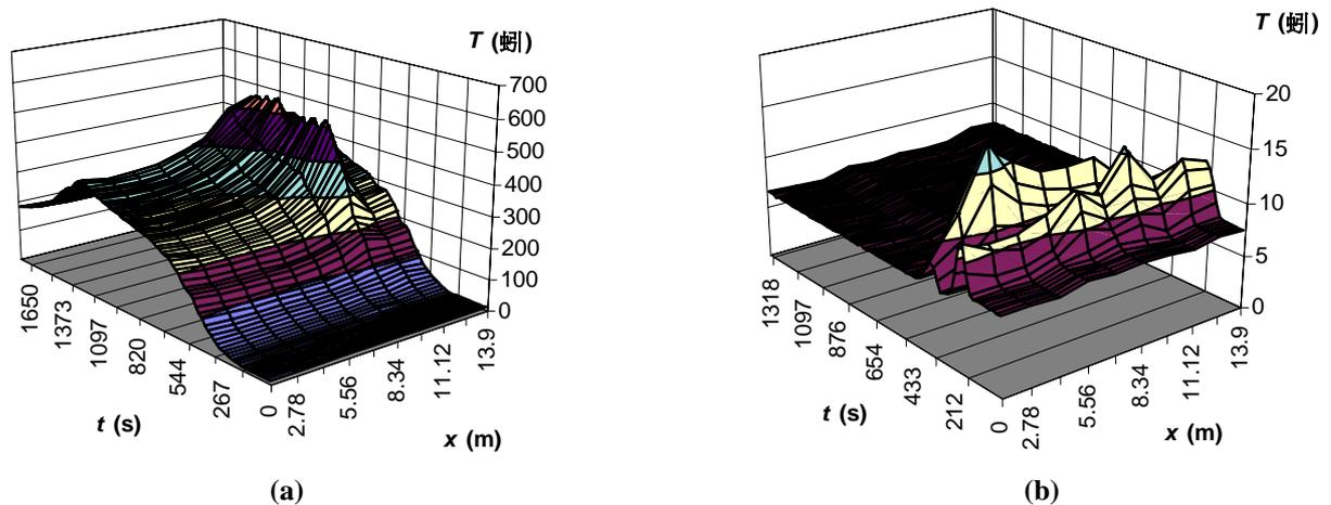
**Fig. 4: Temperature horizontal distribution in the first floor corridor**
