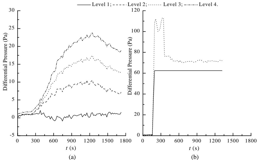
**Fig. 6: Differential pressure distributions in the stairwell during experiments (a) FO4 and (b) FO5**
