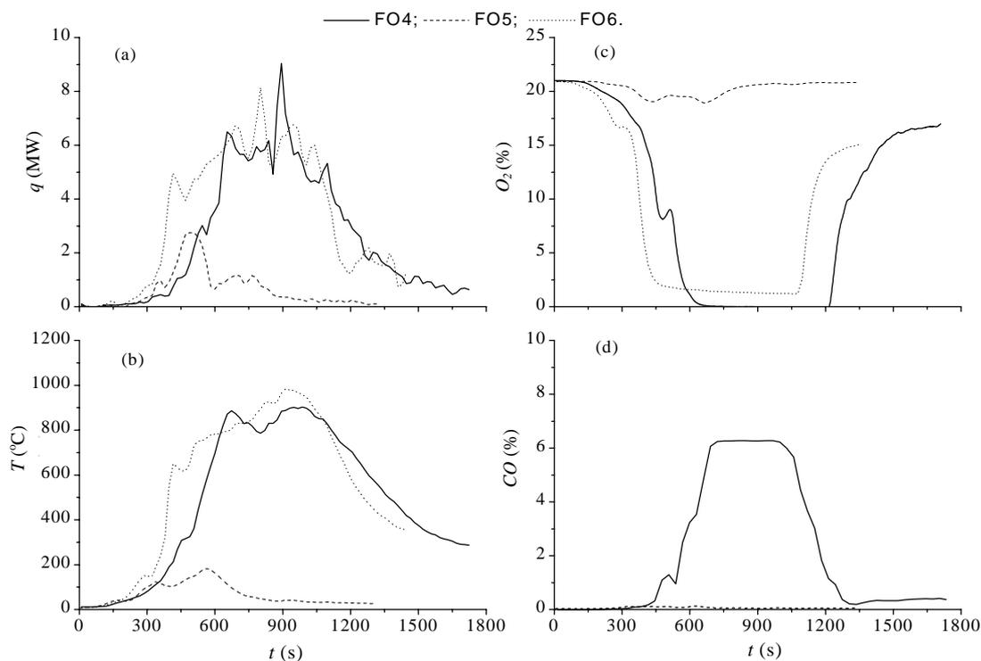
**Fig. 2: Comparison of burn room conditions in experiments FO4, FO5 and FO6**
