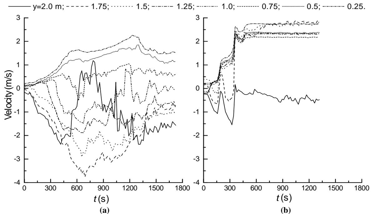
**Fig. 3: Flow velocity distribution at the centre line of the burn room door in experiments (a) FO4 and (b) FO5**
