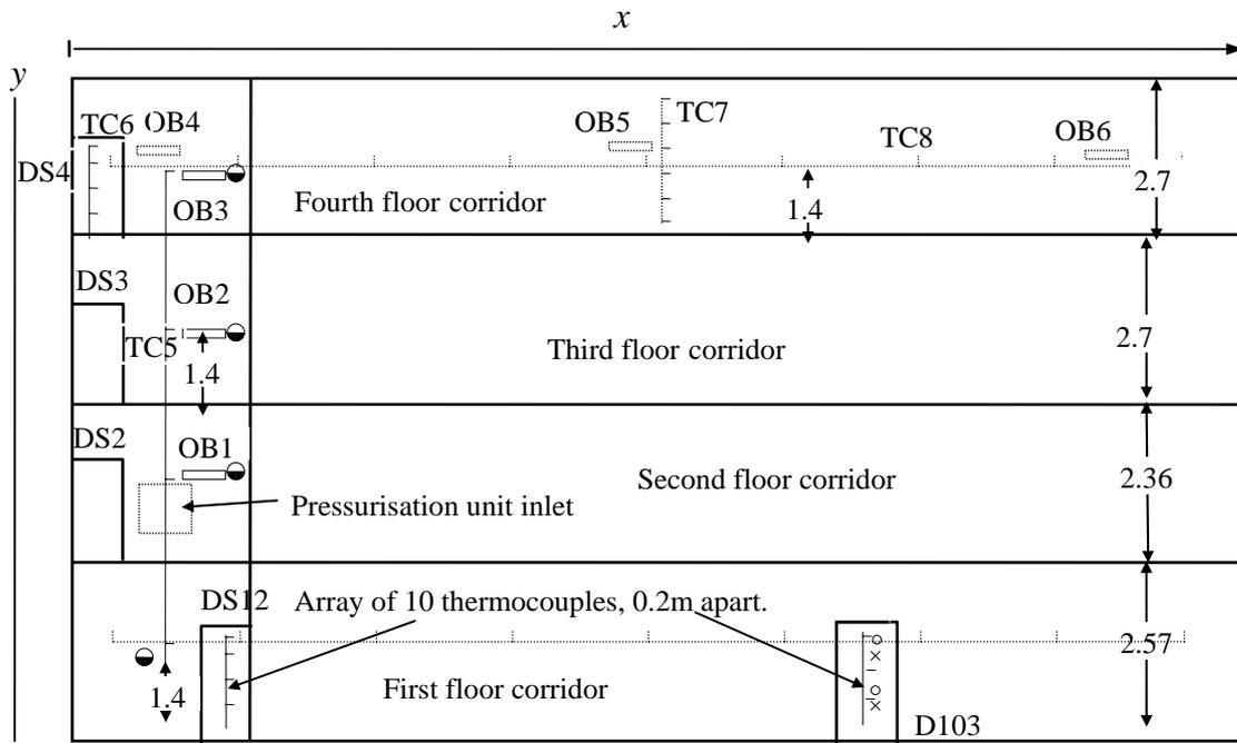
(b) Elevation view of instrumentation layout
