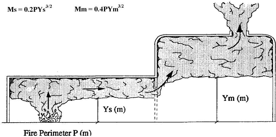
Fig. 4: Entrainment into plume
