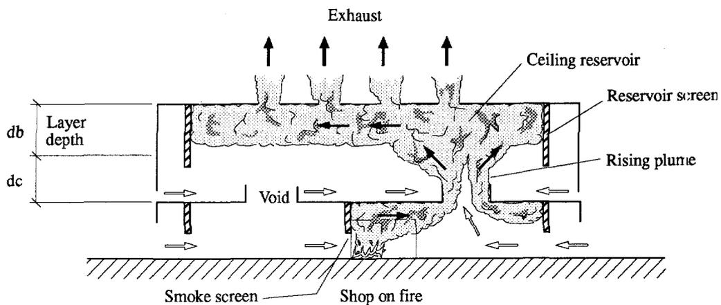
Fig. 7B: Smoke and air movements in two-storey mall with small connecting voids
