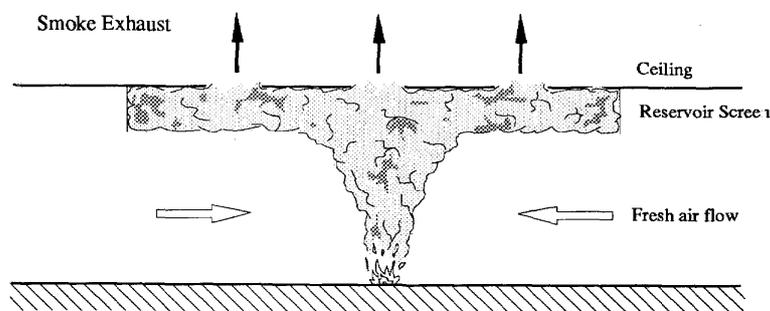
Fig. 2: Principle of system needed to contain smoke in a well-defined layer
