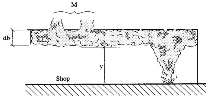
**Fig. 3: Hot smoky gases entering (and being removed from) a ceiling layer**
