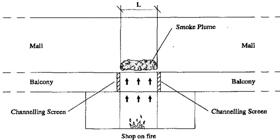
Fig. 5B: The use of smoke channelling screens to produce a compact rising plume
