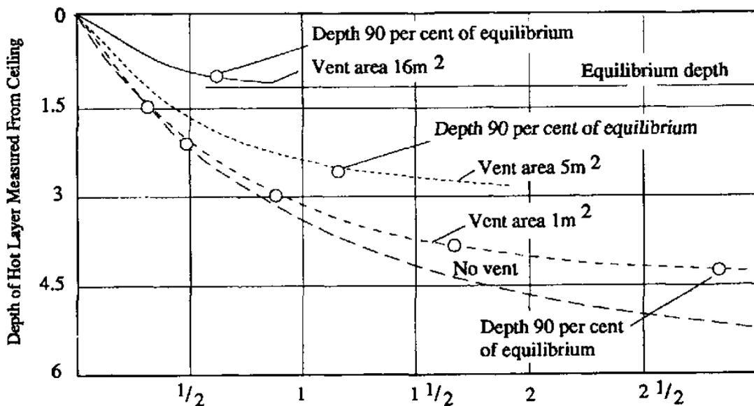
Time for 3m x 3m fire to fill 30m x 30m x 6m building to depth db - min
