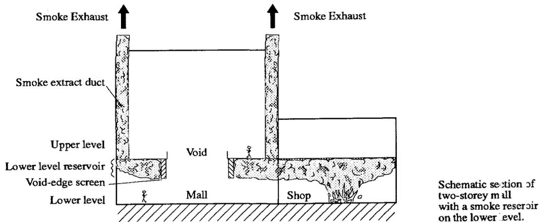
Fig. 6B: Schematic section of two-storey mall with a smoke reservoir on the lower level
