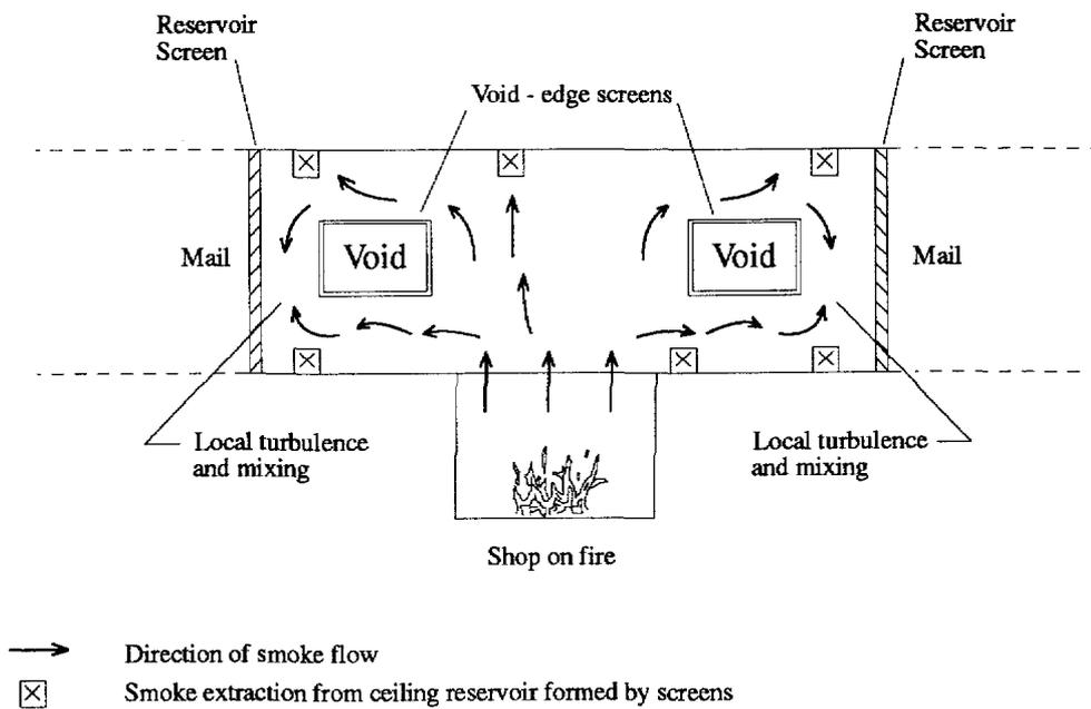
Fig. 6A: Schematic plan of multi-storey mall with a smoke reservoir on each level
