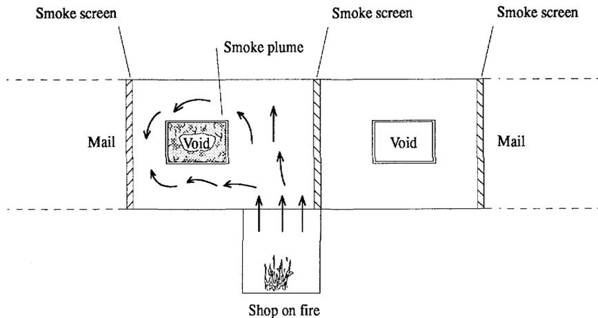
Fig. 7A: Plan view of smoke circulation pattern below upper deck with smoke-restraining screens
