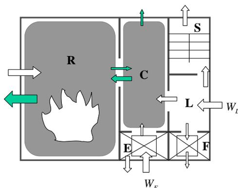
Fig. 12: Vestibule pressurization smoke control
