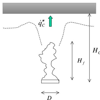
Fig. 4: Ceiling heat transfer from impinging fire plume
