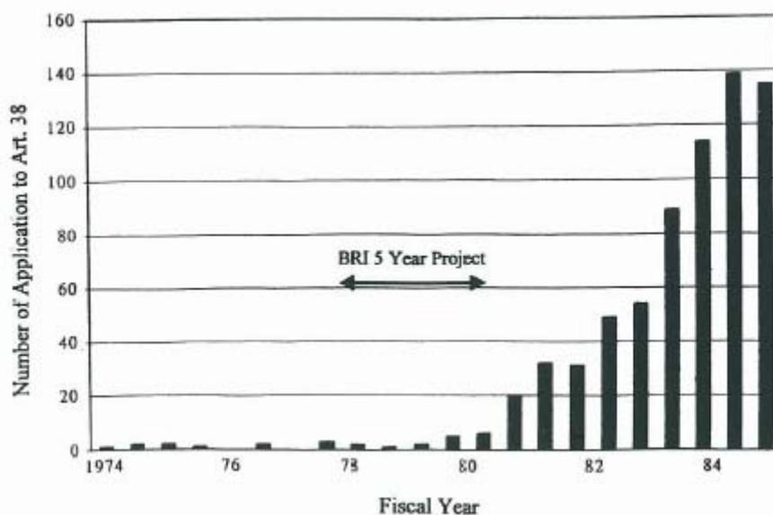
Fig. 1: Growth of number of performance-based fire safety designs of buildings
