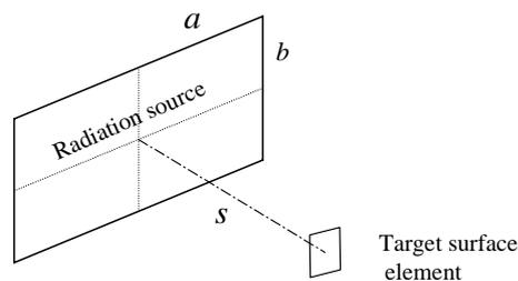
Fig. 14: Calculation of a typical configuration factor
