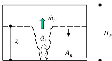
Fig. 10: Smoke filling in a room with t-square fire
