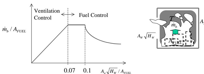
Fig. 13: Mass burning rate in compartment fire
