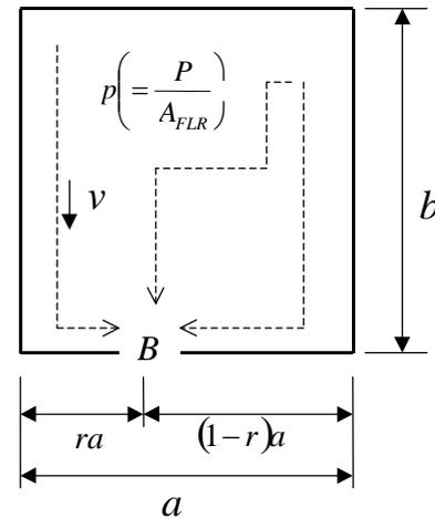
Fig. 5: Evacuation from a room with a single exit
