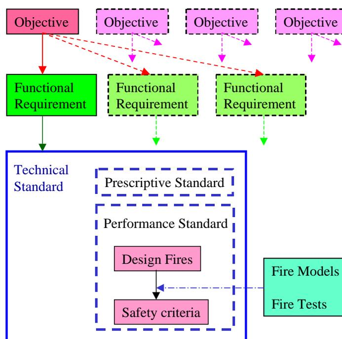
Fig. 2: Framework of a performance-based fire safety design method
