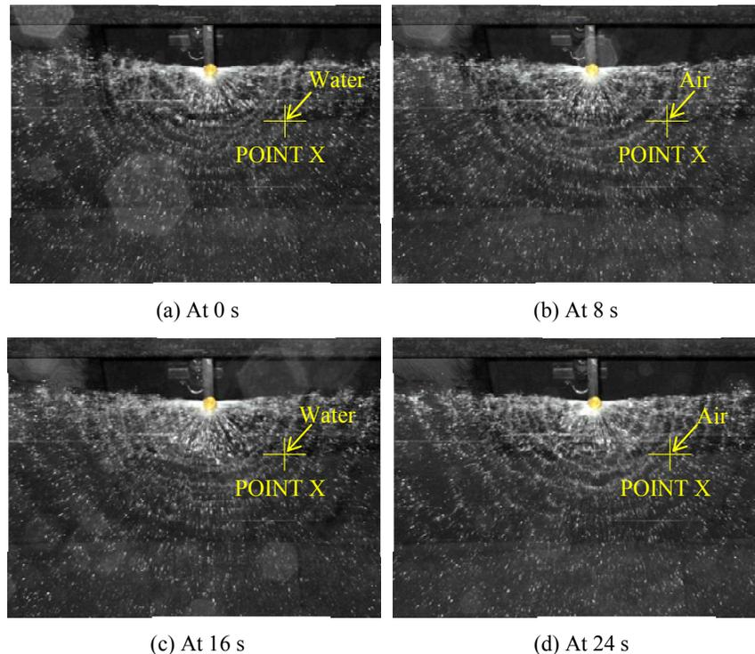
Fig. 1: Transient water curtain pattern
