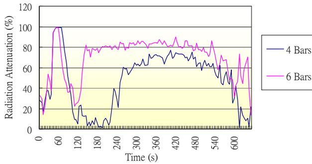
**Fig. 6: Radiation attenuation for fire size of 160 kW under 4 and 6 bars**
