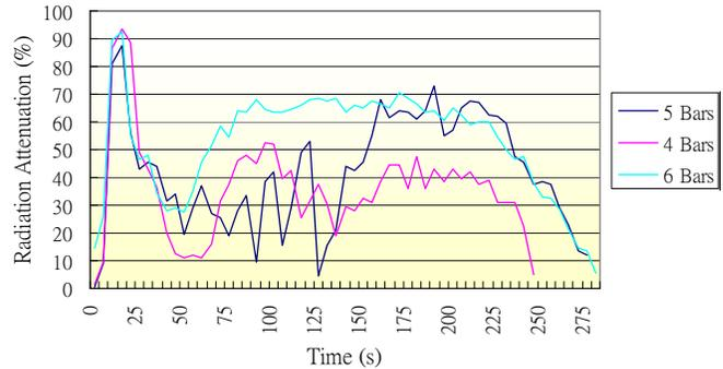
**Fig. 7: Radiation attenuation for fire size of 41 kW under 4, 5 and 6 bars**
