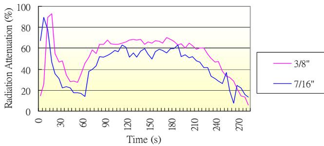
**Fig. 9: Radiation attenuation of two different nozzles under 6 bars working pressure and 1.02 l/s flow rate**
