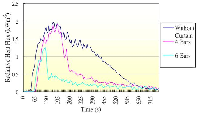
**Fig. 5: Radiative heat flux for fire size of 160 kW**
