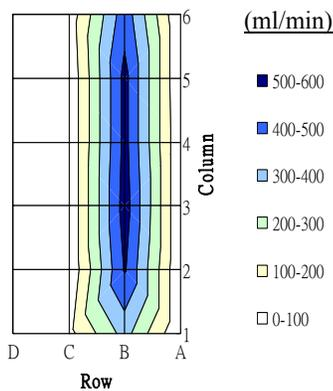
**Fig. 3: Water flow rate distribution of 3/8” drencher head at 4 bars working pressure**
