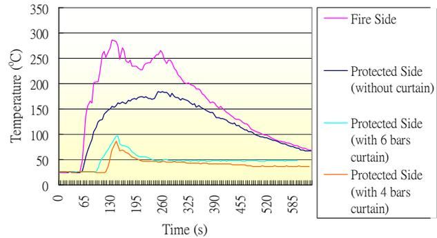
**Fig. 10: Temperature profiles in the fire chambers**
