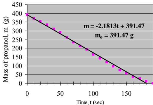
**Fig. 4: Experimental result of mass loss rate (g/s) of propanol**
