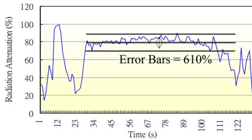
**Fig. 11: Determination of the error bars of the radiation attenuation**
