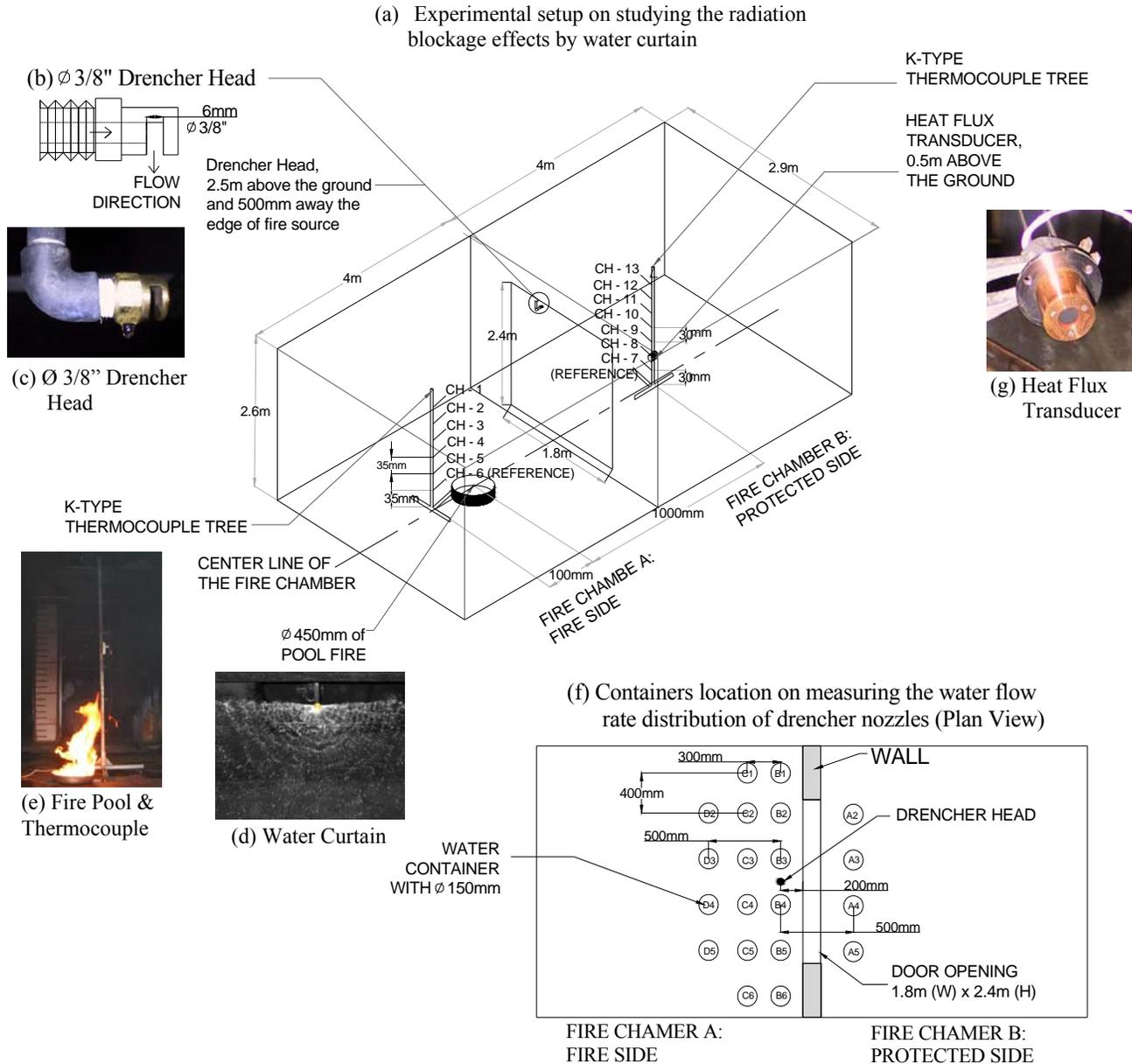
Fig. 2: Experimental setup for studying the radiation blockage effects by water curtain
