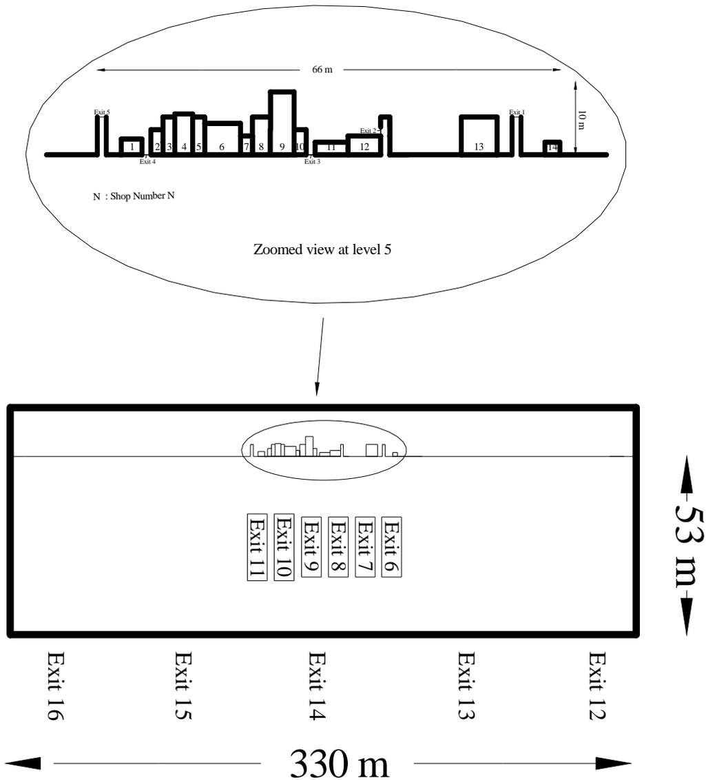
Fig. 2: The layout of arrival level of the Airport Terminal Building
