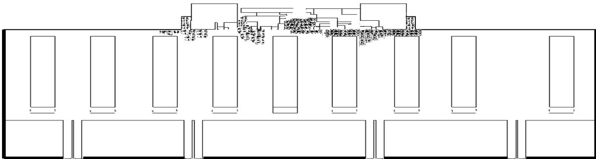
Fig. 4: Evacuation pattern of buildingEXODUS (at time = 40 s)
