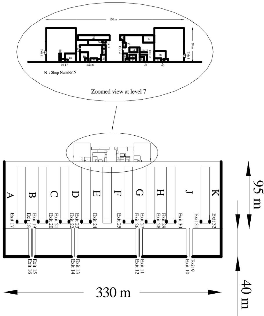
Fig. 1: The layout of departure level of the Airport Terminal Building
