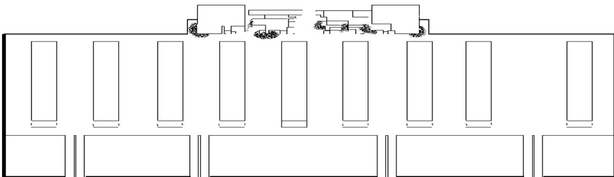
Fig. 5: Evacuation pattern of SIMULEX (at time = 40 s)
