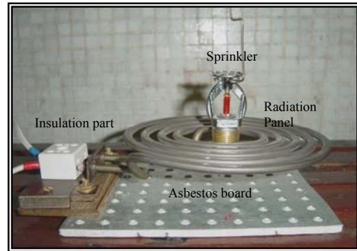
**Fig. 2: Orientation of sprinkler**
