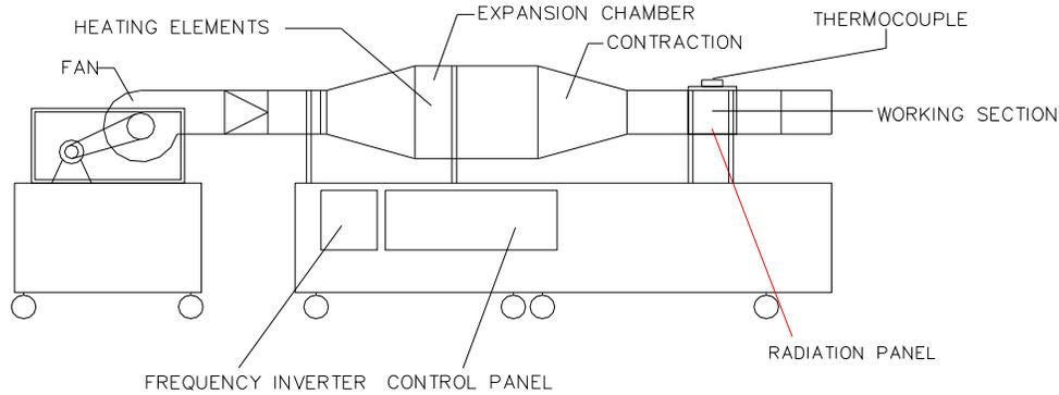
**Fig. 1: BSE wind tunnel**
