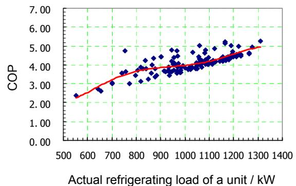
Fig. 5: COP variation with the actual refrigerating load of a single centrifugal unit
