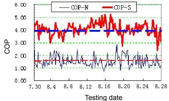
Fig. 4: The actual COP variations with testing time and mean values
