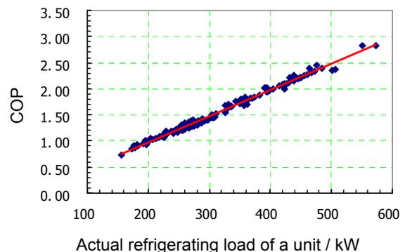
Fig. 6: COP variation with the actual refrigerating load of a single direct-fired unit
