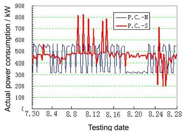
Fig. 1: The total power consumption variations of the north and the south subsystem
