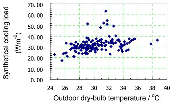
Fig. 3: Actual cooling loads variation with outdoor dry-bulb temperature
