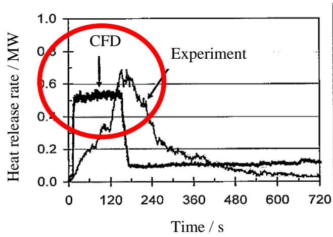
**Fig. 1: A bad example of CFD prediction, Hietaniemi et al. (2004)**
