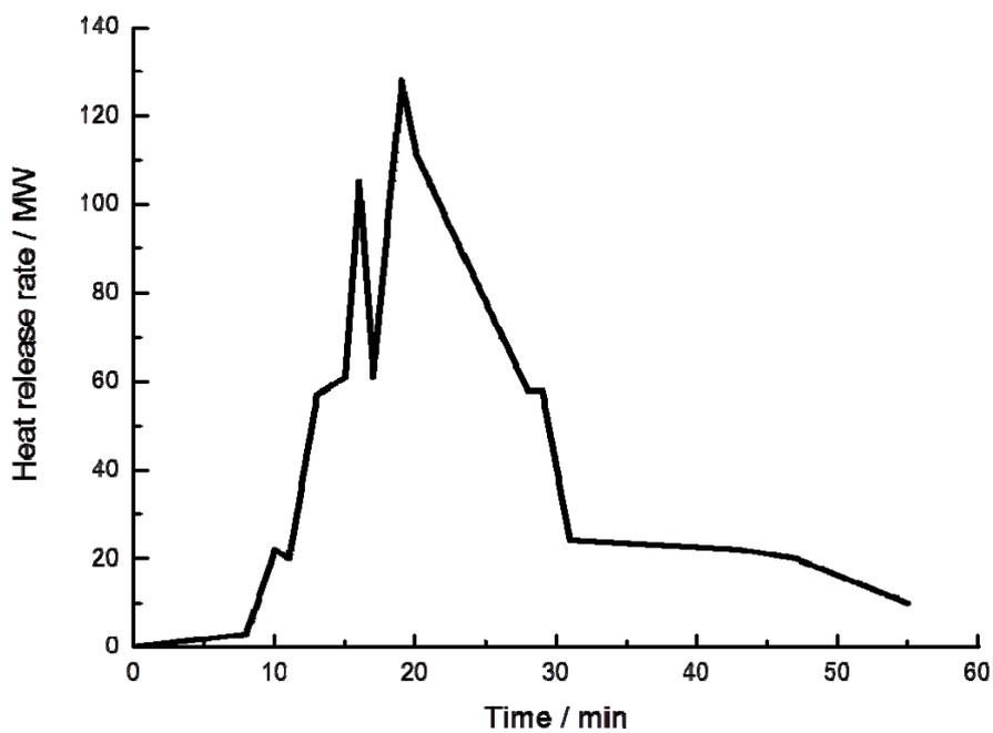
Fig. 2: An HG curve reported by Ingason and Lönnemark (2005)
